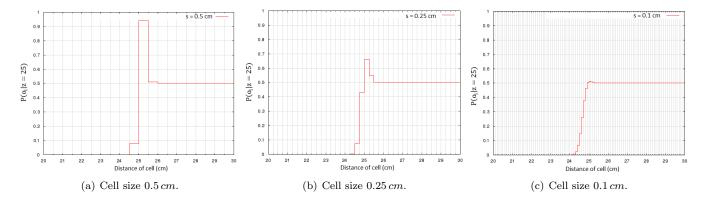
Fig. 3. Influence of the grid resolution on the ISM for  $s_1 = 0.5$  cm (a),  $s_2 = 0.25$  cm (b) and  $s_3 = 0.1$  cm (c). The sensor has a constant precision  $\sigma = 0.2$  cm and senses an obstacle at distance z = 25 cm.
