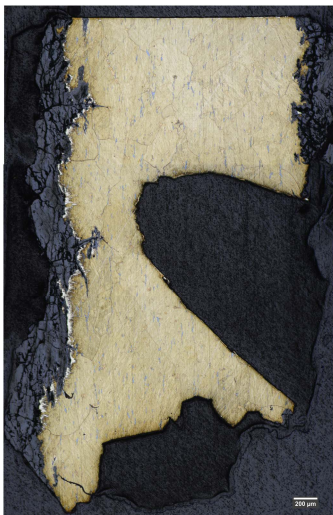
Fig. 11. Bowl SEALIP/TH/KS/5's high-tin bronze microstructure mosaic, showing equiaxed and twinned grains from hot working.
