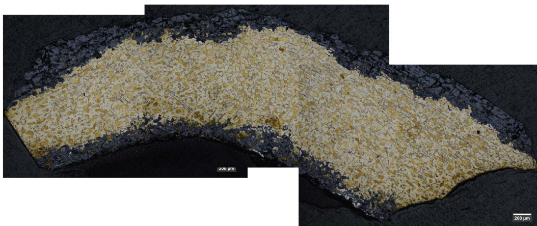
Fig. 9. Bowl SEALIP/TH/KS/3's microstructure mosaic showing characteristic martensitic texture of high-tin bronzes.
