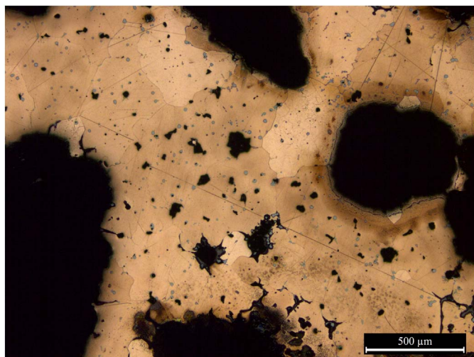
Fig. 8. 'Dong Son drum' SEALIP/TH/KS/2's equi-axed cored microstructure, courtesy of Pira Venunan.
