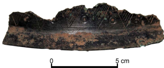
Fig. 4. Fragment of high-tin bronze bowl from Khao Sek, illustrating the shiny patina typical of this alloy, and the incised decoration often seen on wrought and quenched 'Indianising' bowls.
