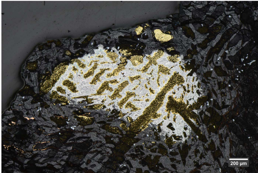
Fig. 6. Casting splash SEALIP/TH/KS/1's partially corroded dendritic microstructure, indicating the metal was left as-cast.
