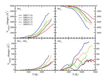
FIG. 9. Volumes of the all  $BO_3$ ,  $BO_4$ ,  $BO_3 + BO_4$  and  $SiO_4$  entities with respect to the temperature in each systemes, display in the left top corner, right top corner, left bottom corner and right bottom corner respectively.
