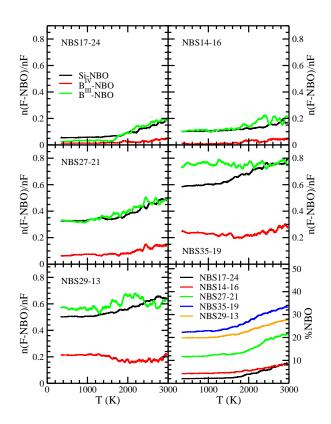
FIG. 5. Number of NBOs close to a network former atom F with F = Si,  $B^{IV}$  and  $B^{III}$  (respectively the black, red and green lines) normalized by the number of such atoms. Bottom right panel: percentage of NBOs in all the NBS systems.
