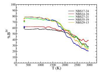
FIG. 4. Amount of four-fold coordinated boron atoms during the quenching for different NBS compositions. The stars are the experimental results at room temperature  $^{44,55}$ .
