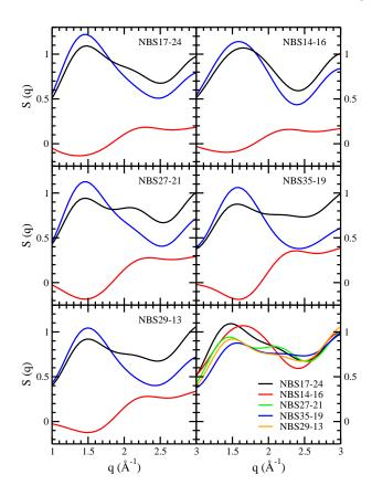
FIG. 3. The total neutron structure factors (black curve) are splitted into two contributions: one arising from the partial structure factors involving Na atoms (red) and one involving all the others interactions (blue). The whole set of total neutron structure factors is also given in the right bottom panel.
