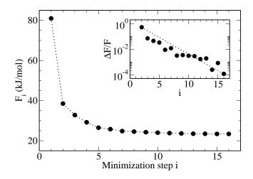
Figure 1. Convergence of the free energy estimation during the minimization process for a CO<sub>2</sub> molecule in water with a box size L = 24 Å, N = 72 and  $n_{max} = 3$ . The inset shows the evolution of the relative difference in the free energy functional between successive steps.
