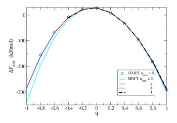
Figure 6. Solvation free energy of a hypothetical  $CH_4^q$  molecule calcultated by MDFT-HNC as a function of its charge q for different angular resolution  $n_{max} = 2$  to 5. The finite size corrections of equations 38 and 39 are included. For comparison, we also show the exact 1D-IET results that can be calculated for this spherically symmetric case.
