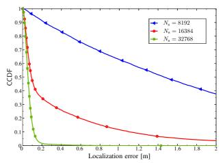
Fig. 8. Complementary cumulative distribution function (CCDF) of the localization error for different number of pulses per symbol.
