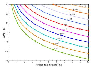
Fig. 7. SQNR at the ADC output.
