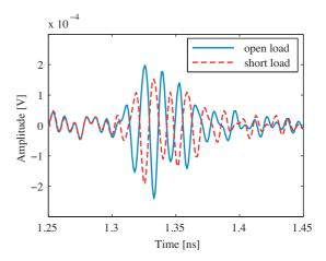
Fig. 4. Example of the backscattered signal for tag open and short circuit loads (only the antenna mode component is shown).
