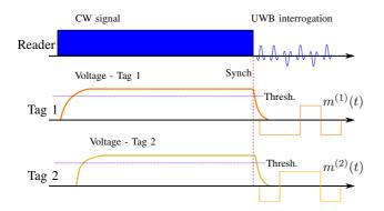
Fig. 5. Wake-up synchronization scheme and signaling.
