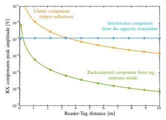
Fig. 6. Typical dynamic range of a UWB-RFID system.
