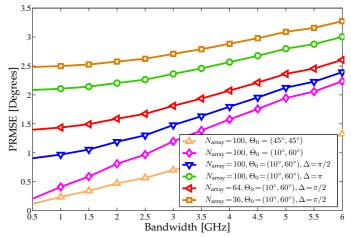
Fig. 6: PRMSE vs. bandwidth for different values of  $N_{\rm array}$ , different steering angles and in presence/absence of quantization effects.
