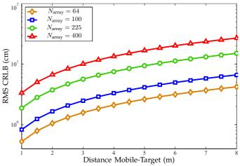
Fig. 4: RMS CRLB vs. mobile-target distance for different values of  $N_{\text{array}}$ ,  $\Theta_0 = (45^\circ, 45^\circ)$ , and W = 500 MHz.
