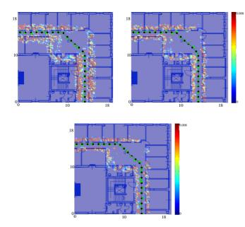
Fig. 11: 2D mapping using  $4 \times 4$  (top-left),  $10 \times 10$  (top-right) and  $15 \times 15$  (bottom) antenna arrays and with quantization and mobile position (10 cm) and orientation errors (5°).
