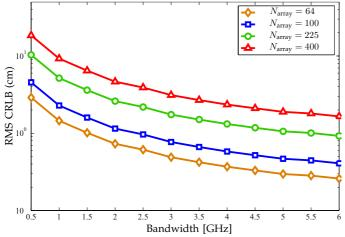
Fig. 5: RMS CRLB vs. transmitted signal bandwidth W for a mobile-target distance of 10 m, and for  $\Theta_0 = (45^\circ, 45^\circ)$ .
