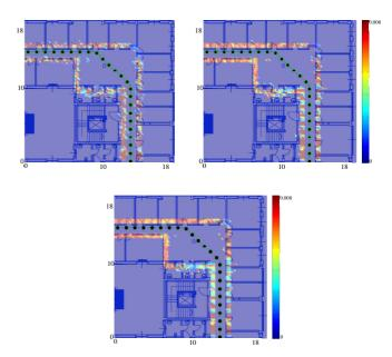
Fig. 9: 2D mapping using  $10 \times 10$  antenna arrays with W = 500 MHz (top-left), W = 2 GHz (top-right) and W = 3 GHz (bottom) with no quantization errors and a perfect knowledge of mobile position.
