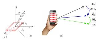
Fig. 2: Array structure (a) and beam pointing error scheme (b).
