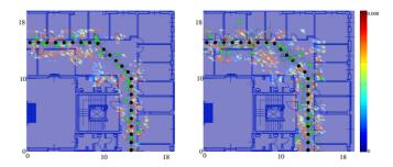
Fig. 14: 2D mapping using  $10 \times 10$  antenna arrays with position and mobile orientation errors  $0.5 \text{ m}+20^{\circ}$  (left) and  $1 \text{ m}+20^{\circ}$  (right) and W = 1GHz.
