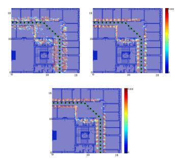
Fig. 10: 2D mapping using  $4 \times 4$  (top-left),  $10 \times 10$  (top-right) and  $15 \times 15$  (bottom) antenna arrays with a perfect knowledge of mobile position and with array quantization errors.
