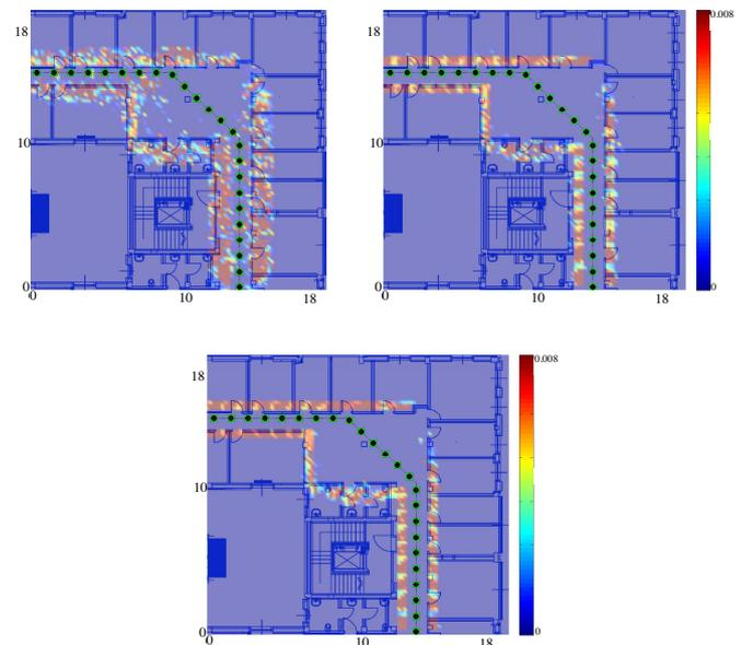
Fig. 10: 2D mapping using  $4 \times 4$  (top-left),  $10 \times 10$  (top-right) and  $15 \times 15$  (bottom) antenna arrays with a perfect knowledge of mobile position and with array quantization errors.
