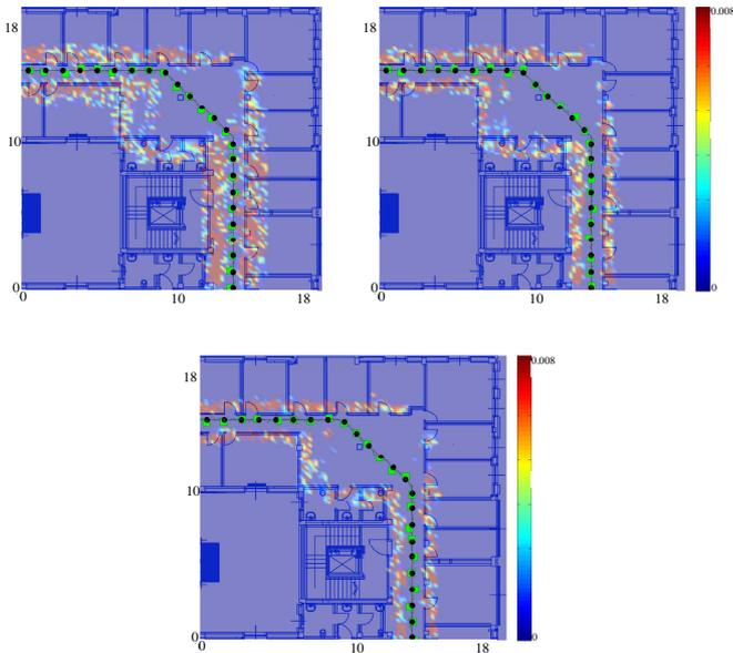
Fig. 11: 2D mapping using  $4 \times 4$  (top-left),  $10 \times 10$  (top-right) and  $15 \times 15$  (bottom) antenna arrays and with quantization and mobile position (10 cm) and orientation errors ( $5^\circ$ ).
