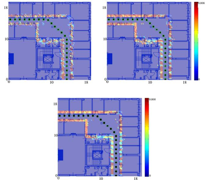
Fig. 9: 2D mapping using  $10 \times 10$  antenna arrays with  $W = 500$  MHz (top-left),  $W = 2$  GHz (top-right) and  $W = 3$  GHz (bottom) with no quantization errors and a perfect knowledge of mobile position.
