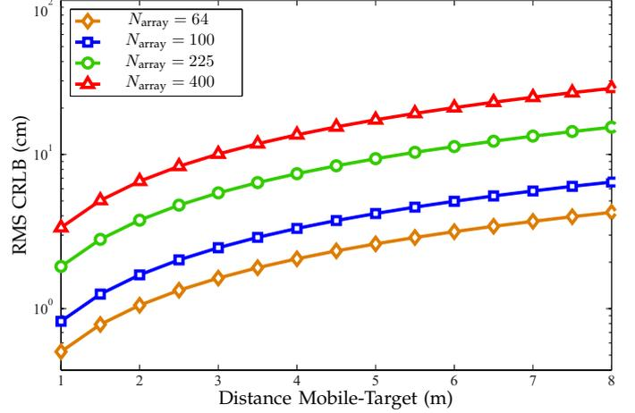
Fig. 4: RMS CRLB vs. mobile-target distance for different values of  $N_{\text{array}}$ ,  $\Theta_0 = (45^\circ, 45^\circ)$ , and  $W = 500$  MHz.
