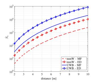
Fig. 5. Required number of pulses for different receiver architectures.
