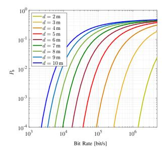
Fig. 6. Obtained data rates for different reader-tag distances.
