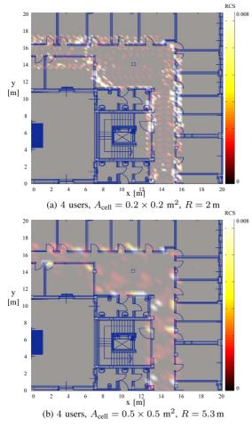
Fig. 7. Reconstructing map using the receiver A, different sized grid cells and radar maximum range conditions.
