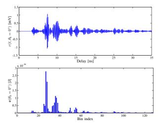
Fig. 5. Accumulated received signal using the receiver A and energy profile using the receiver B over  $N_{\rm p}=100$  pulses.
