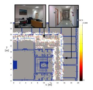
Fig. 8. Reconstructed map using the receiver B, 4 users, a grid cell area of  $A_{\text{cell}} = 0.2 \times 0.2 \text{ m}^2$  a radar maximum range of R = 2 m.
