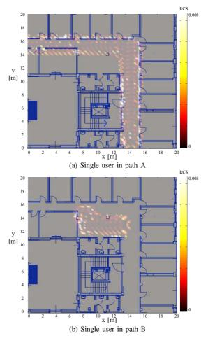
Fig. 6. Reconstructing map using by different users using the receiver A,  $A_{\rm cell} = 0.2 \times 0.2$  m<sup>2</sup>, R = 2 m.
