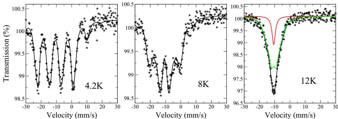
Fig. 13. <sup>151</sup>Eu Mössbauer spectra at selected temperatures in EuIrGe<sub>3</sub>, in the equal moment phase (4.2 K), close to the equal moment incommensurate transition (8 K) and close to the incommensurate-paramagnetic transition (12 K). At 12 K, the green subspectrum represents the incommensurate pattern and the red subspectrum the paramagnetic pattern. (For interpretation of the references to color in this figure caption, the reader is referred to the web version of this paper.)
