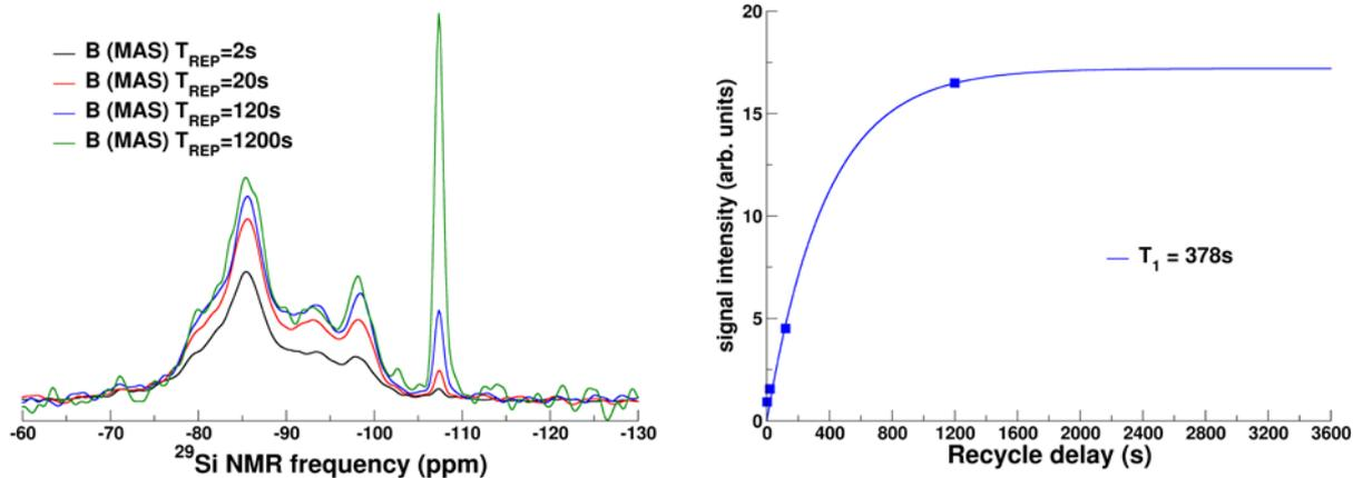
**Figure SI5-1.** (Left) Evolution of the  $^{29}\text{Si}$  NMR spectra with the recycle delay for a sample similar to the ones studied in the present work. (Right) Intensity of the quartz peak (around -108 ppm) plotted as a function of the recycle delay.
