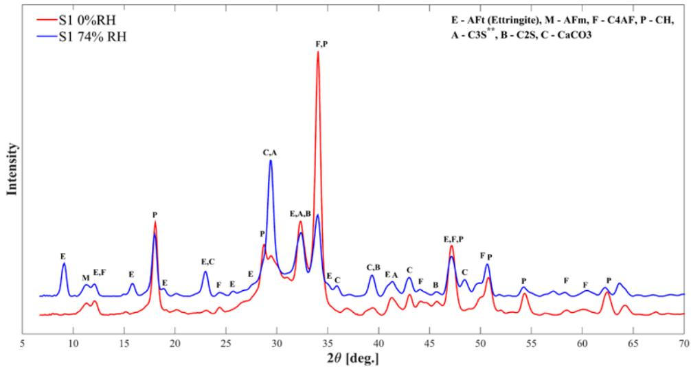
**Figure SI2-1.** Qualitative analysis of the X-ray ( $\text{Cu } K\alpha_1=1.540598 \text{ \AA}$ ) powder diffraction results obtained on S1 hydrated cement paste equilibrated at 0% RH (red) and 74% RH (blue). Samples aged 28 days. To make the comparison with literature data easier, the diagrams, recorded with a molybdenum anode ( $\lambda_{K\alpha_1} = 0.70932 \text{ \AA}$ ), were then calculated with respect to a copper anode ( $\lambda_{K\alpha_1} = 1.540598 \text{ \AA}$ ).
