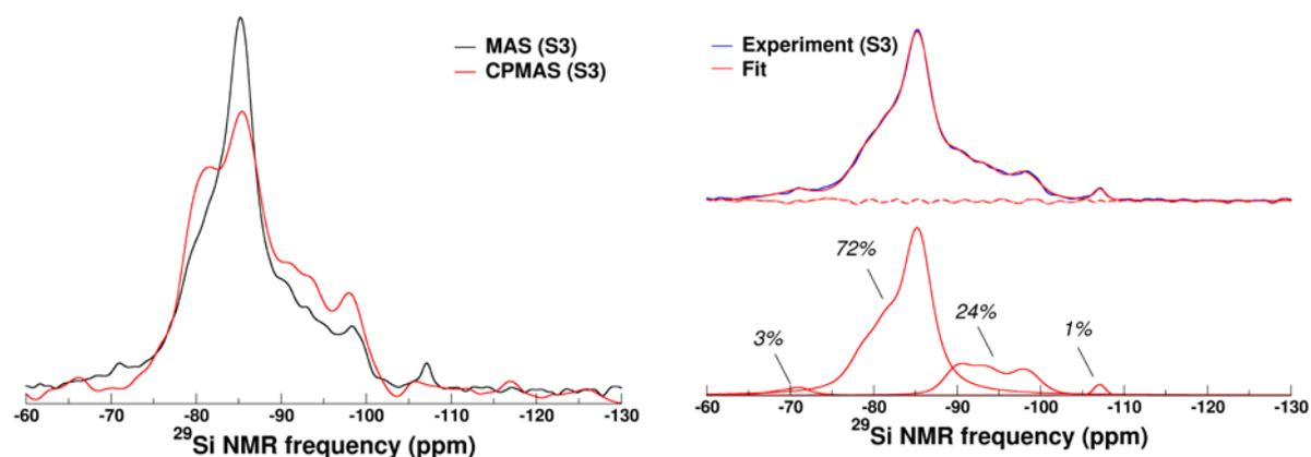
**Figure SI5-4.** Comparison between  $^{29}\text{Si}$  MAS NMR and CP-MAS NMR spectra (left) for S3 equilibrated at 11% RH. Experimental (blue line) and simulated (red line) for the  $^{29}\text{Si}$  MAS NMR spectra (right).
