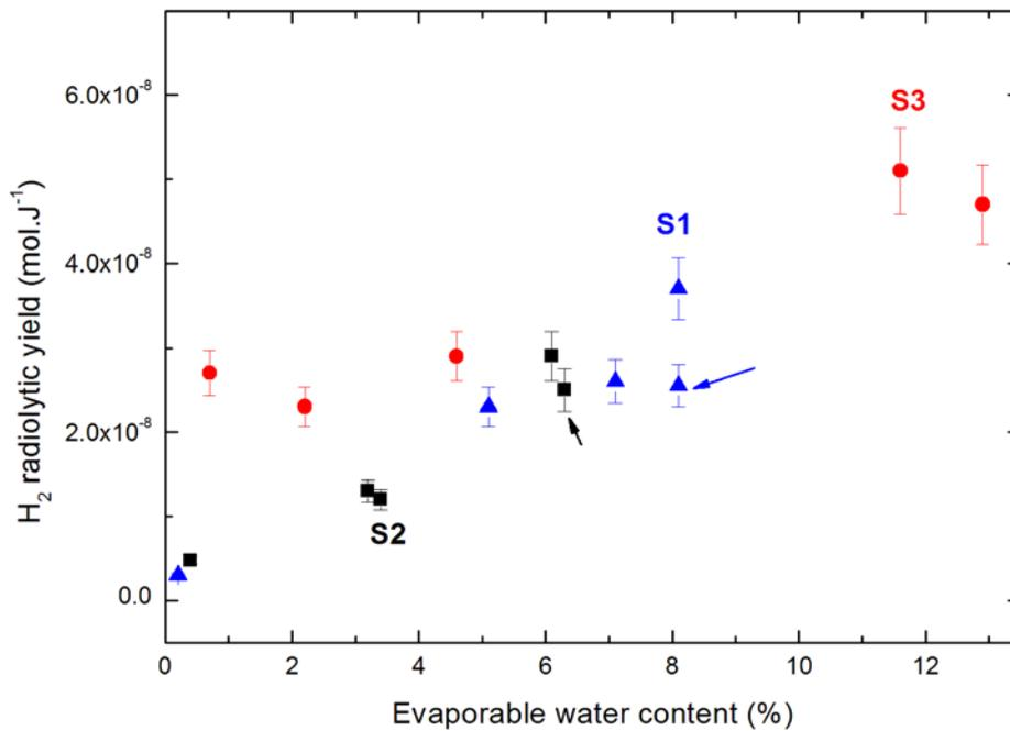
**Figure SI7-1.** Evolution of the H<sub>2</sub> radiolytic yield with the evaporable water content for S1 (blue triangles), S2 (black squares) and S3 (red circles). The arrows highlight the effect of the high calcite content for S1 and S2 at 74% RH.
