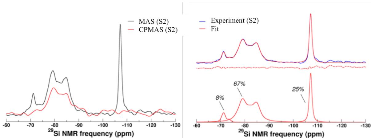
**Figure SI5-3.** Comparison between  $^{29}\text{Si}$  MAS NMR and CP-MAS NMR spectra (left) for the S2 sample equilibrated at 11% RH. Experimental (blue line) and simulated (red line)  $^{29}\text{Si}$  MAS NMR spectra (right). The red dashed line represents the error.
