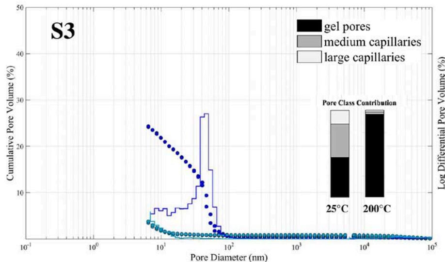
**Figure SII-1.** Pore size distribution of the sample S3 before (dark blue) and after (light blue) hydrothermal exposure measured with mercury intrusion (MIP). Pore classification after ref. [1].
