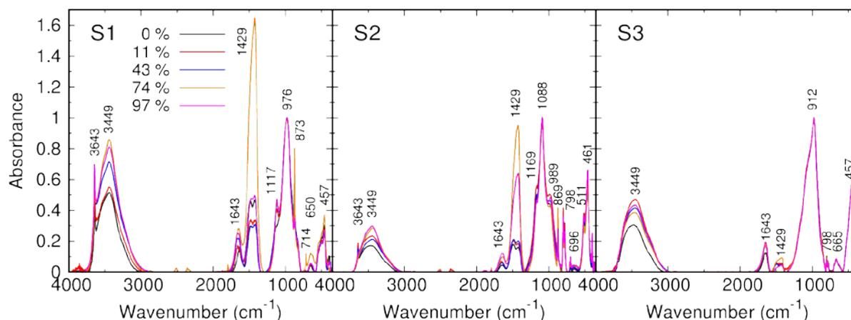
**Figure SI3-1.** Infrared spectra for all samples. The spectra are normalized with respect to the band around 970-1100  $\text{cm}^{-1}$ , which corresponds to Si-O stretching vibrations.
