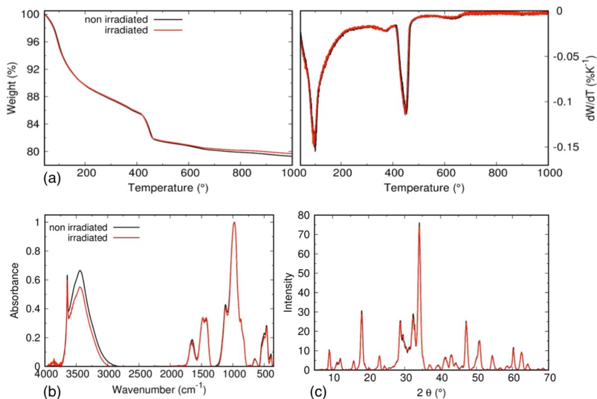
**Figure SI6-1.** S1 sample equilibrated at 11% RH before (in black) and after irradiation (red) at 200 kGy characterized by different techniques: a) TGA curves (left) and DTA curves (right); b) infrared spectroscopy and c) XRD analysis. Concerning the IR spectra, the discrepancy observed in the O-H stretching region (3000-4000 cm<sup>-1</sup>) is due to the preparation of the pellets and is not significant.
