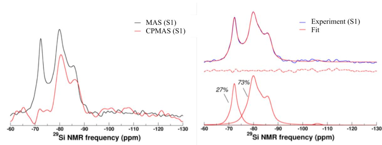
**Figure SI5-2.** Comparison between  $^{29}\text{Si}$  MAS NMR and CP-MAS NMR spectra (left) of S1 equilibrated at 11% RH. Experimental (blue line) and simulated (red line)  $^{29}\text{Si}$  MAS NMR spectra (right). The red dashed line represents the error.
