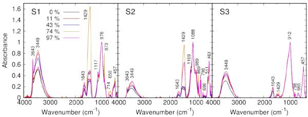
**Figure SI3-1.** Infrared spectra for all samples. The spectra are normalized with respect to the band around 970-1100 cm<sup>-1</sup>, which corresponds to Si-O stretching vibrations.
