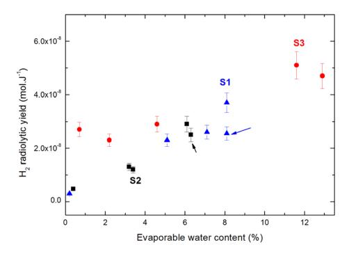
**Figure SI7-1.** Evolution of the  $H_2$  radiolytic yield with the evaporable water content for S1 (blue triangles), S2 (black squares) and S3 (red circles). The arrows highlight the effect of the high calcite content for S1 and S2 at 74% RH.
