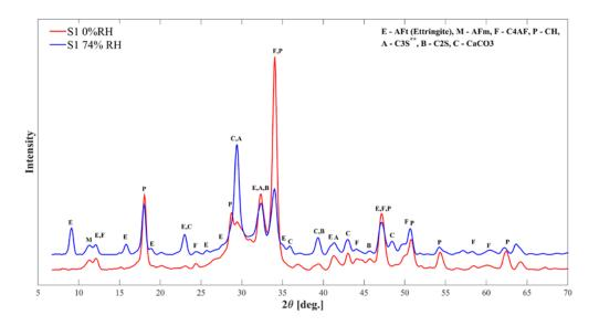
**Figure SI2-1.** Qualitative analysis of the X-ray (Cu K $\alpha_1$ =1.540598 Å) powder diffraction results obtained on S1 hydrated cement paste equilibrated at 0% RH (red) and 74% RH (blue). Samples aged 28 days. To make the comparison with literature data easier, the diagrams, recorded with a molybdenum anode ( $\lambda K_{\alpha 1} = 0.70932$  Å), were then calculated with respect to a copper anode ( $\lambda K_{\alpha 1} = 1.540598$  Å).
