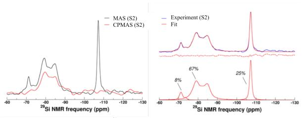
**Figure SI5-3.** Comparison between <sup>29</sup>Si MAS NMR and CP-MAS NMR spectra (left) for the S2 sample equilibrated at 11% RH. Experimental (blue line) and simulated (red line) <sup>29</sup>Si MAS NMR spectra (right). The red dashed line represents the error.
