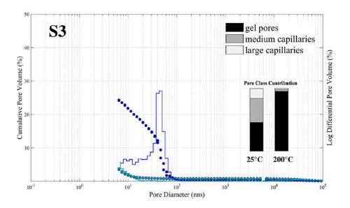
**Figure SI1-1.** Pore size distribution of the sample S3 before (dark blue) and after (light blue) hydrothermal exposure measured with mercury intrusion (MIP). Pore classification after ref. [1].
