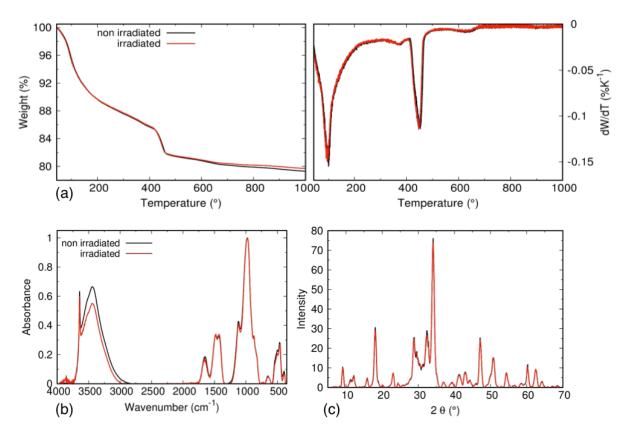
**Figure SI6-1.** S1 sample equilibrated at 11% RH before (in black) and after irradiation (red) at 200 kGy characterized by different techniques: a) TGA curves (left) and DTA curves (right); b) infrared spectroscopy and c) XRD analysis. Concerning the IR spectra, the discrepancy observed in the O-H stretching region (3000-4000 cm<sup>-1</sup>) is due to the preparation of the pellets and is not significant.
