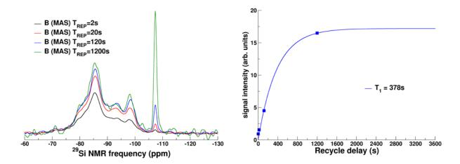
**Figure SI5-1.** (Left) Evolution of the <sup>29</sup>Si NMR spectra with the recycle delay for a sample similar to the ones studied in the present work. (Right) Intensity of the quartz peak (around -108 ppm) plotted as a function of the recycle delay.
