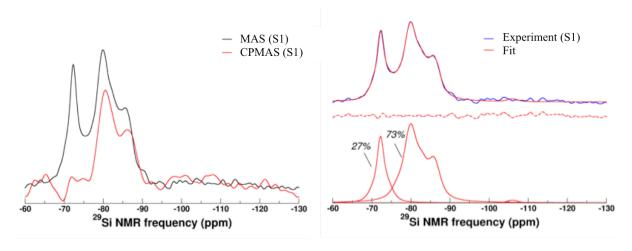
**Figure SI5-2.** Comparison between <sup>29</sup>Si MAS NMR and CP-MAS NMR spectra (left) of S1 equilibrated at 11% RH. Experimental (blue line) and simulated (red line) <sup>29</sup>Si MAS NMR spectra (right). The red dashed line represents the error.
