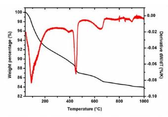
Figure SI4-1. TGA (in black) and the differential curve (DTG, in red) curves of S2 at 11% RH.
