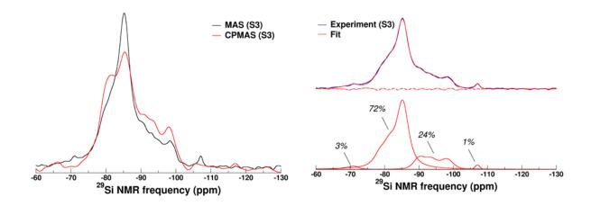
**Figure SI5-4.** Comparison between <sup>29</sup>Si MAS NMR and CP-MAS NMR spectra (left) for S3 equilibrated at 11% RH. Experimental (blue line) and simulated (red line) for the <sup>29</sup>Si MAS NMR spectra (right).
