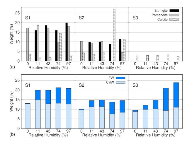
Fig. 1. Mass percentage (a) of the main phases (ettringite, portlandite and calcite) and (b) of water (evaporable water, EW; and chemically bound water, CBW) as determined from TGA measurements in samples SI 4 as a function of relative humidity. The mass percentage of ettringite has been approximately evaluated (see Supporting Information SI 4). The error bars are estimated to be 15% in all cases except ettringite for which the error bar is even larger. The amount of ettringite is difficult to
