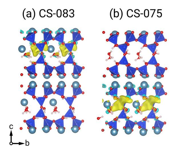
**Fig. 4.** Details of: (a) The spin density for the CS-083 model with an excess electron. (b) The spin density for the CS-075 model with an excess electron. Isosurfaces of positive and negative spin densities ( $\pm 0.002 \text{ e.A}^{-3}$ ) are represented in yellow and blue, respectively. In both cases the structures have been optimized at the M06-2X level.
