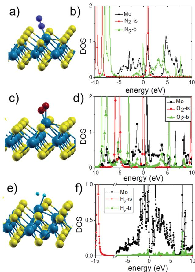
Fig. 7 Equilibrium geometry of different adsorbed molecules on a defective MoS<sub>2</sub> monolayer (a) N<sub>2</sub>, (c) O<sub>2</sub> and (e) H<sub>2</sub>. In (b), (d) and (f) the DOS of the Mo atom (black square) bonded to each molecule (green triangles) are shown together with the DOS of the isolated molecule for N<sub>2</sub>, O<sub>2</sub> and H<sub>2</sub>, respectively. The Fermi energy is fixed at 0 eV.
