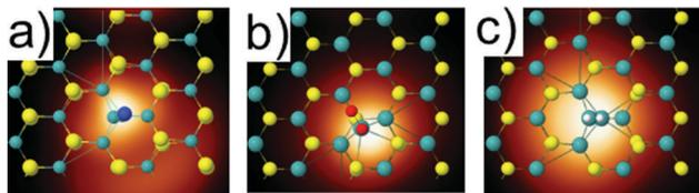
Fig. 8 Simulated STM image at voltage  $V = -1.0$  V for (a)  $N_2$ , (b)  $O_2$  and (c)  $H_2$  on their corresponding most attractive defect.
