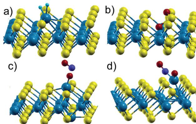
Fig. 9 Atomic representation of the dissociative configurations of different molecules on a defective  $MoS_2$  monolayer: (a)  $H_2$  dissociated on the substitutional Mo atom occupying a S vacancy, (b)  $O_2$  molecule dissociated in a Mo vacancy, (c)  $NO_2$  over two Mo atoms occupying the S-divacancy and (d)  $NO_2$  over a Mo substitutional atom on a S vacancy.
