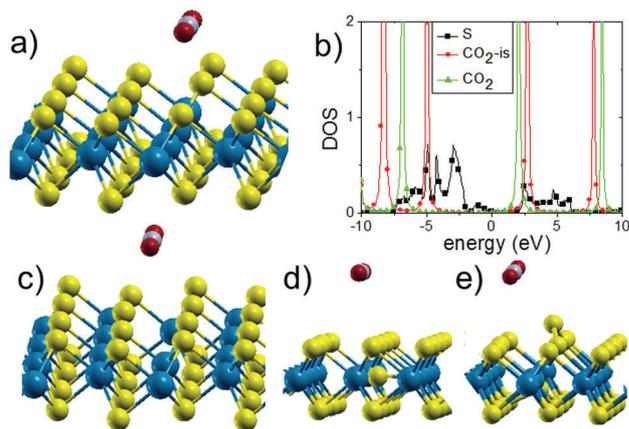
**Fig. 3** Equilibrium geometry of a CO<sub>2</sub> molecule physisorbed on a MoS<sub>2</sub> monolayer with (a) S vacancy, (c) Mo vacancy, (d) and (e) one and two S substitutional atoms occupying a Mo vacancy; (b) DOS of a S atom far away from the vacancy (black squares), the CO<sub>2</sub> placed over the S vacancy (green triangles) and the isolated molecule (red circles). The Fermi energy is fixed at 0 eV.
