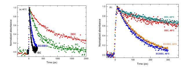
**Figure 3.** (a) Normalized decay kinetics at 46°C of the solvated electron in DEC (red circles), PC (green squares), EC (black down triangles) and EC/DEC (blue up triangles); (b) comparison of the normalized decay kinetics at 46°C and at room temperature (22°C). The lines guide the eyes.
