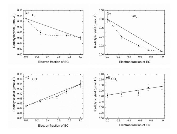
**Figure 6.** Effect of the EC electron fraction on the radiolytic yields of the main decomposition gases quantified by  $\mu$ GC. (a) H<sub>2</sub>; (b) CH<sub>4</sub>; (c) CO; (d) CO<sub>2</sub>. The uncertainty bars are estimated to 10 %.
