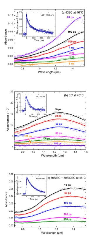
**Figure 1.** Transient optical absorption spectra in (a) DEC; (b) EC and (c) 50/50 EC/DEC mixture after the picosecond electron pulse (dose per pulse: 47 Gy). Kinetics is given in the
