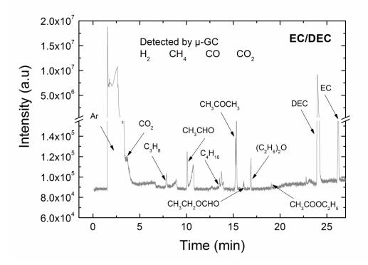
**Figure 4.** Gas decomposition products of EC/DEC identified by GC-EI/MS after  $\gamma$ -irradiation at 20 kGy. The formation of acetone can be due to washing and not to irradiation.
