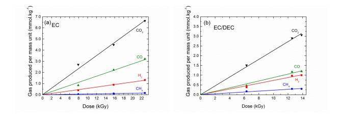
**Figure 5.** Evolution of the main decomposition products formed in the gas phase and measured by  $\mu$ -GC after  $\gamma$ -irradiation of EC (a) and EC/DEC (b) as a function of the dose.
