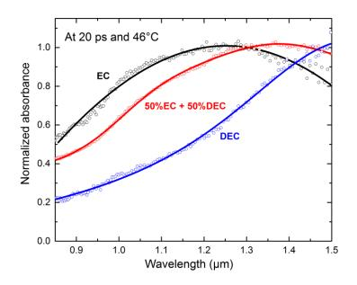
**Figure 2.** Normalized spectra, measured at 46°C, of the solvated electron in EC (black), DEC (blue) and 50/50 EC/DEC (red) measured 20 ps after the electron pulse. The circles are the experimental points and the lines are a guide for the eyes.
