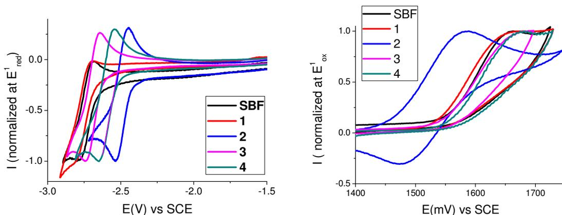
**Figure 5.** Cyclic Voltammetry (CV) of **1-4** and **SBF** recorded in DMF/ $\text{Bu}_4\text{NPF}_6$  0.1 M (reduction, left) and in dichloromethane/ $\text{Bu}_4\text{NPF}_6$  0.2 M (oxidation, right). Sweep-rate: 100 mV/s. Platinum working electrode. All CVs are normalized at the peak potential of the reduction (left) or oxidation (right) process.
