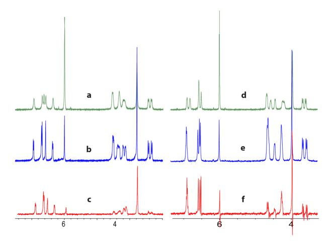
S11: <sup>1</sup>H NMR spectra of compounds **3a** (left) and **3s** (right) for the degassed solutions (spectra a and d); in the presence of xenon (spectra b and e). <sup>129</sup>Xe-<sup>1</sup>H SPINOE spectra of compounds **3a** (spectrum c) and **3s** (spectrum f). The antiphase signals are not SPINOE, but artefacts due to bad subtraction.
