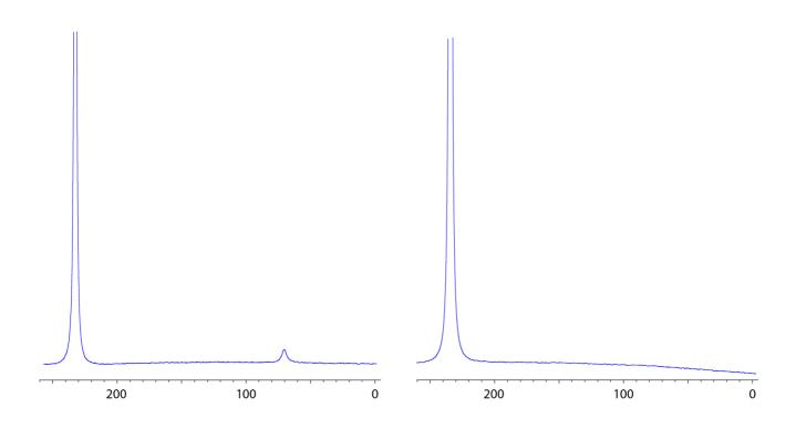
S10: <sup>129</sup>Xe NMR spectra of compounds **3a** (left) and **3s** (right) at 293K
