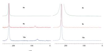
**Figure 2.** One-scan <sup>129</sup>Xe NMR spectra of the samples of **6** (**a** and **s**), **9** (**a** and **s**), **12** (**a** and **s**). The subscripts a and s refer to *anti* and *syn* arrangement of the linkers. Spectra have been recorded at 11.74 T and 293 K. Each sample contained 0.3 +- 0.03 mg of cryptophane (0.4 - 0.5 mM) in 600  $\mu$ L of 1,1,2,2-tetrachloroethane-d<sub>2</sub> and *ca.* 10 mg of xenon (representing a concentration of ca. and mM).
