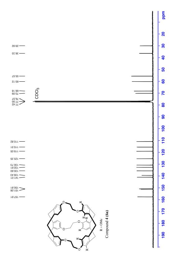
S2: <sup>13</sup>C NMR (75.5 MHz) spectrum of compound (4)-6a in CDCl<sub>3</sub> solution at 298 K.
