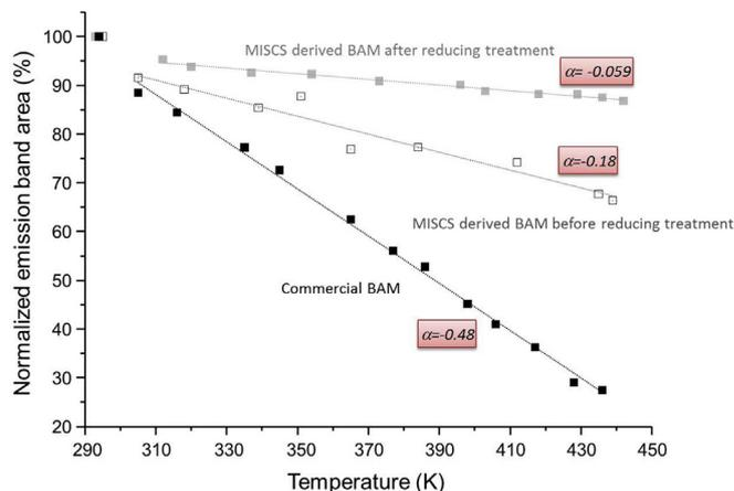
**Fig. 10.** Evolution with temperature of the normalized emission band area of BAM:Eu powders upon a 365 nm LED excitation: commercial and MISCS-derived BAM:Eu powders. Dot lines represent linear fits of the evolutions with corresponding slopes  $\alpha$ .
