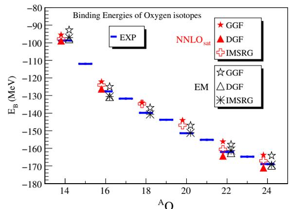
FIG. 1. Oxygen binding energies. Results from SCGF (DGF and GGF) and IMSRG calculations with EM and NNLO<sub>sat</sub> are displayed along with experimental data.
