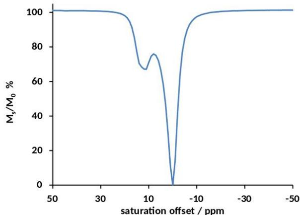
Figure 2: CEST spectrum of the europium complex EuL (19.9 mM; pH 7.4), recorded in H<sub>2</sub>O/D<sub>2</sub>O (95/5 (v/v)) at 400 MHz. The saturation time was 3 s and the saturation power was  $B = 1030$  Hz.
