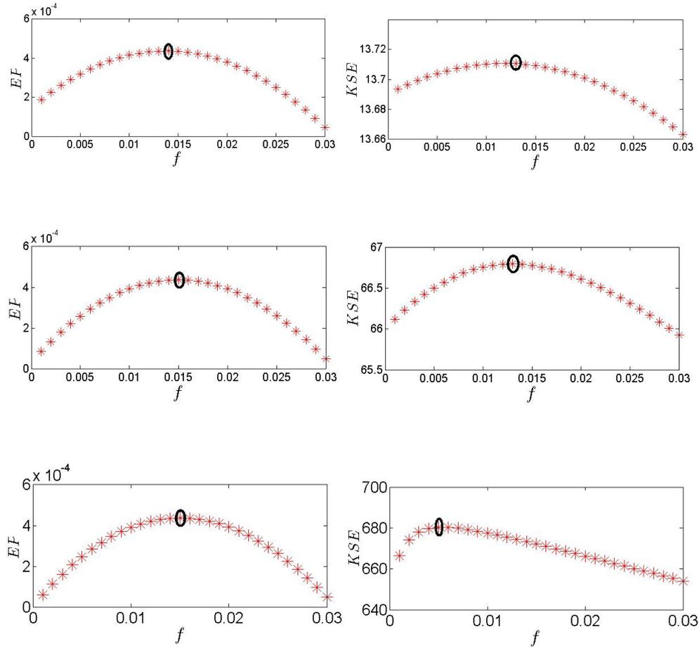
**Figure 1.** Entropy production calculated using Eq. (11) (left) and KS entropy calculated using Eqs. (7) and (15) (right) as functions of  $f$  for  $s = 0.13$  and respectively  $N = 20$ ,  $N = 100$  and  $N = 1000$ .
