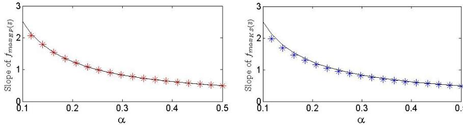
**Figure 5.**  $f_{\max_{KS}(\bar{s})}$  (left) and  $f_{\max_{EP}(\bar{s})}$  (right) as functions of  $\alpha$  and in black the curve  $f(\bar{s}) = \frac{1}{4\alpha}\bar{s}$ . Note that the approximation  $f_{\max_{KS}(\bar{s})} \approx f_{\max_{EP}(\bar{s})} \approx \frac{1}{4\alpha}\bar{s}$  is good.
