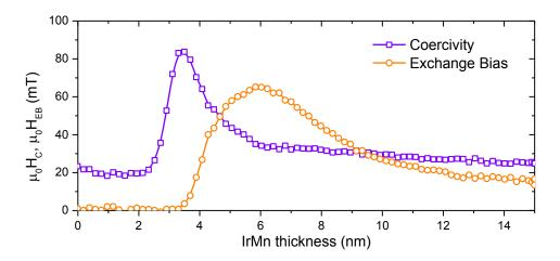
Figure S9: graphs of the exchange bias  $H_{\rm EB}$  and coercive field  $H_{\rm c}$  as a function of IrMn thickness in a Ta (3) / Pt (4) / Co (1.5) / IrMn (0-15) / Pt (2) wedge sample, measured along the out-of-plane direction after annealing in the out-of-plane direction at 225°C in a 0.2 T magnetic field for 30 minutes. The sample shows close to 100% remanence across the entire IrMn thickness range.
