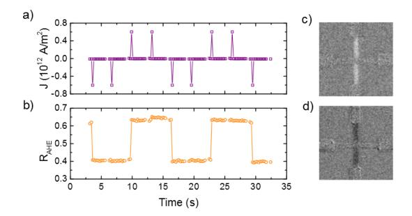
Figure S12: proof-of-principle measurement in a Ta (0.5) / Pt (4) / Co (1.25) / IrMn (6) / TaOx (1.5) sample, demonstrating that a) a train of current pulses produces b) magnetization switching as expected from the SHE. Kerr microscopy images show the magnetization after switching to c) the up-state and d) the down-state.
