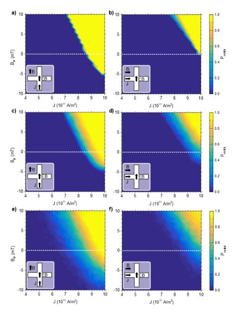
Figure S16: simulated switching probability  $P_{\text{switch}}$  as a function of current density *J* and magnetic field  $B_{\text{ip}}$  along the current direction, in the presence of a,b) a uniform 5 mT EB, c,d) a 5 mT EB with angular spread, and e,f) a  $\chi_3$ -distributed EB with angular spread. For each  $(J,B_{\text{ip}})$  point,  $P_{\text{switch}}$  is computed by averaging over 256 simulations.
