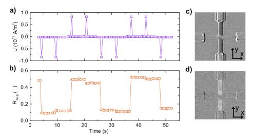
**Figure 2: Switching by current pulses. a)** Applied current density pulse pattern, and **b**) resulting anomalous Hall resistance. Switching is observed for one current polarity in either state, without any applied magnetic field. Differential Kerr microscopy images of the microwire after switching to **c**) the low  $R_{AHE}$  state and **d**) the high  $R_{AHE}$  state confirm the magnetization reversal.
