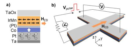
**Figure 1: Schematic sample layout. a)** Cross section of the deposited stack, showing the magnetic easy axis of the Co (white arrow), simplified spin structure of the IrMn (thick black arrows), exchange bias field (orange arrow), and spin current generated from a charge current running through the Pt (circles). **b)** Hall cross structure consisting of two 10 x 1  $\mu$ m rectangles, and measurement scheme.
