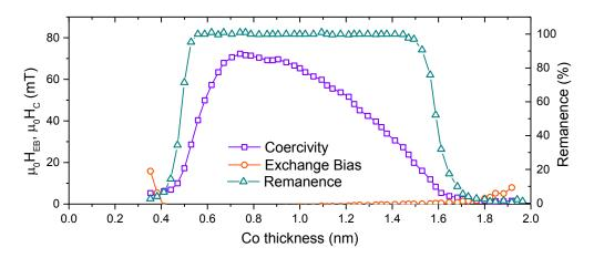
Figure S8: graphs of the exchange bias *H*<sub>EB</sub>, coercive field *H*<sub>c</sub>, and remanence as a function of cobalt thickness in a Ta (3) / Pt (3) / Co (0-2) / Pt (0.3) / IrMn (6) / Pt (3) wedge sample, measured using polar MOKE in the out-of-plane direction after annealing in the in-plane direction at 225°C in a 2T magnetic field for 30 minutes.
