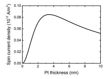
Figure S10: spin current density as a function of Pt thickness, computed for constant total current  $I_e$ . Spin diffusion and current shunting effects are taken into account using simple models. The optimum Pt thickness is found to be between 3 and 4 nm.
