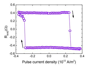
Figure S13: anomalous hall resistance  $R_{AHE}$  of a Ta(4)/Pt(3)/Co(1.2)/Ta(5) microwire, recorded while sweeping the applied pulse current density from high negative values to high positive values and back under application of a -10 mT magnetic field along the current flow direction. Sudden magnetization reversal is observed at a critical current density below  $3 \cdot 10^{11}$  A/m<sup>2</sup>.
