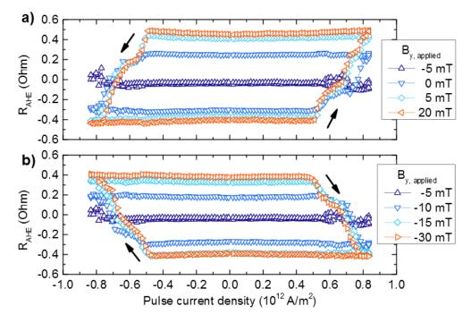
**Figure 3:** Current density sweeps. Anomalous Hall resistance  $R_{AHE}$  measured during pulse current density sweeps for various applied in-plane magnetic fields. The magnetic field enhances deterministic **a**) upward and **b**) downward switching. The arrows indicate the sweep direction.
