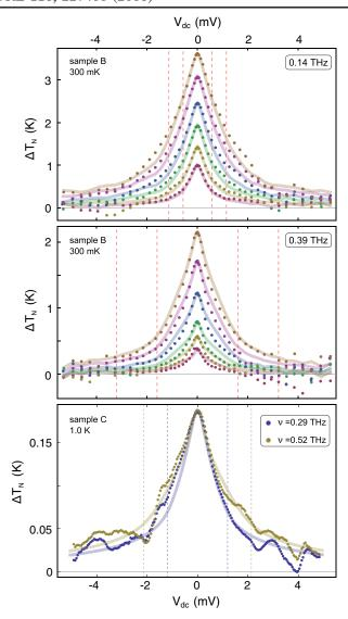
FIG. 3. Top and central panels: noise difference  $\Delta T_N$  for  $\nu=0.14$  and 0.39 THz, measured at 300 mK on sample B. In both,  $V_{\rm em}$  is changed from 8 (dark purple) to 13 V (dark yellow). Bottom panel:  $\Delta T_N$  measured at 1 K on sample C for  $\nu=0.29$  (blue) and 0.52 THz (dark yellow) and  $V_{\rm em}=13$  V. In all panels, symbols are the experimental data, and continuous lines are fits combining heating and PASN, as explained in Fig. 2.
