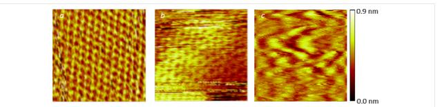
**Figure 1:** Structural characterization of the substrates. STM images ( $2.3 \times 2.3 \text{ m}^2$ ) of a HOPG surface (a) and CVD monolayer graphene transferred onto a fused quartz plate (b:  $2.3 \times 2.3 \text{ m}^2$  and c:  $50 \times 50 \text{ m}^2$ ). The images were acquired under air atmosphere, in the height (constant current) mode. The setpoint current was  $I_S$  = 100 pA, and the bias was  $V_T$  = 200 mV. The height scale is also shown for graphene on quartz (c).
