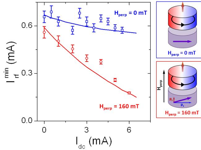
FIG. 3. **Reducing  $I_{\text{rf}}^{\text{min}}$  by compensation of damping.** The d.c. current dependence of  $I_{\text{rf}}^{\text{min}}$  for two magnetic fields,  $H_{\text{perp}} = 0$  and 160 mT and  $\theta_{\text{H}} = 90.1^\circ$ , where the data points are the experimental data and the line is the fit with Eq. 1
