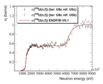
FIG. 4. The  $^{238}$ U(n, f) cross section obtained with the small diameter targets: U8c as target and U5c (black points) and U5b as reference targets. The ENDF/B VII-1 [23] evaluation is shown for comparison. The results are given with a resolution of 50 bins / decade and the error bars correspond to the statistical uncertainties only.
