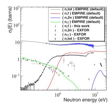
FIG. 11. The calculated cross sections for the main neutron-induced reaction channels of  $^{237}$ Np, with the code EMPIRE and the default parameters of the models chosen, in the energy range 100 keV to 20 MeV, along with the corresponding experimental data from the EXFOR database [1]. The results for the (n,tot),  $(n,\gamma)$ , (n,f), and (n,2n) reaction channels are shown, the latter two exhibiting significant differences compared to the experimental data.
