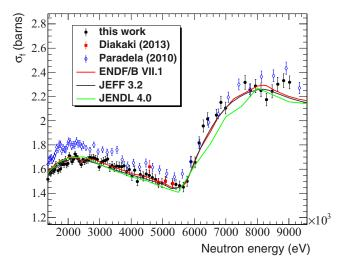
FIG. 7. The  $^{237}$ Np(n, f) cross section, shown with 50 bins/decade, in the neutron energy range 1.5–9 MeV. The error bars correspond to the statistical uncertainties. The present data are compared to the experimental data of Paradela [3] (obtained from the same facility) and Diakaki [2] (obtained with the same target at another neutron production facility as explained in the text), and the evaluations ENDF/B-VII.1 [23], JEFF 3.2 [25], and JENDL 4.0 [24].
