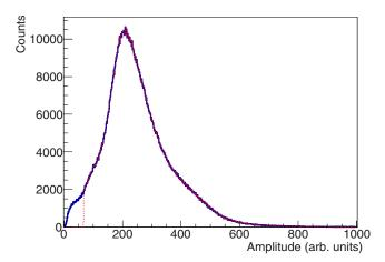
FIG. 2. The FF amplitude distribution from the pulse shape analysis of the <sup>237</sup>Np target. The blue curve corresponds to the analysis without additional threshold for the exclusion of low amplitude pulses, and the red dotted line corresponds to the amplitude distribution with the threshold chosen as discussed in Sec. III A.
