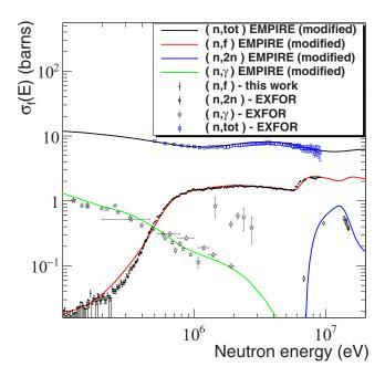
FIG. 12. The calculated cross-sectional results for the main neutron-induced reaction channels on <sup>237</sup>Np, with the code EMPIRE and modified parameters as explained in the text, in the energy range 100 keV to 20 MeV, along with the corresponding experimental data found in the EXFOR database [1]. A good agreement with the experimental data was obtained.
