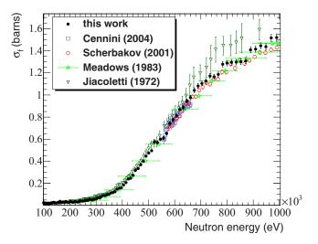
FIG. 8. Comparison of the present data with selected data from the EXFOR database [1], in the neutron energy range 100 keV to 1 MeV.
