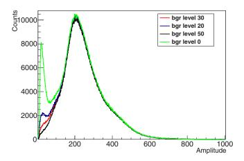
FIG. 3. The histograms of the FF amplitude distributions obtained with different choices of the background level, from the pulse shape analysis of the Np7 target data.
