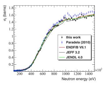
FIG. 6. The  $^{237}$ Np(n, f) cross section, shown with 50 bins / decade, in the neutron energy range 100 keV to 1.5 MeV. The error bars correspond to the statistical uncertainties. The relative statistical uncertainty did not exceed 3% above 500 keV. The present results are compared to the latest experimental data of Paradela [3] (obtained from the same facility) and to the evaluations ENDF/B-VII.1 [23], JEFF 3.2 [25], and JENDL 4.0 [24].
