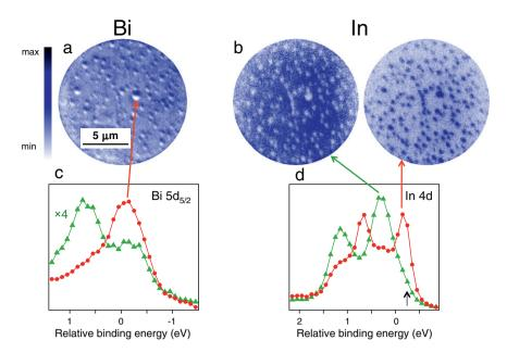
**Fig. 6.** 30 BL Bi/lnAs(111)B sample after 10 min annealing at 300 °C: (a) Bi PEEM image averaged over the whole Bi  $5d_{5/2}$  photoelectron spectrum; (b) In PEEM image recorded at the energy of the intensity maximum of the In 4d photoelectron spectrum, between the clusters (left) and on the clusters (right); (c) and (d) Bi  $5d_{5/2}$  and In 4d core level spectra for two regions: between the Bi clusters (green curve with triangles) and on the Bi clusters (red curve with dots).
