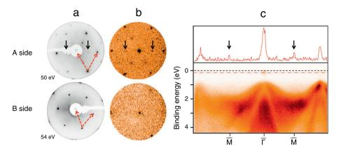
Fig. 1. Clean InAs(111): (a) LEED patterns (at 50 eV for the A side and at 54 eV for the B side). The basis vectors of the reciprocal space are shown as dashed (red) arrows; (b)  $\mathbf{k}$ -maps near the Fermi level; (c) ARPES of the A side along the  $\overline{\Gamma}$ - $\overline{M}$  direction (bottom panel) and intensity profile of the ARPES spectrum near (red dash-dotted line) the Fermi level (black dashed line) (top panel).
