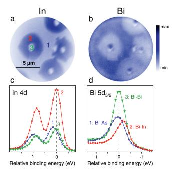
**Fig. 5.** 30 BL Bi/lnAs(111)A sample after a 10 min annealing at 300 °C: (a) In 4d and (b) Bi 5d PEEM images; (c) In 4d and (d) Bi  $5d_{5/2}$  photoelectron spectra corresponding to the regions 1, 2 and 3 of (a).
