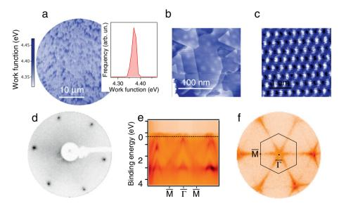
**Fig. 2.** 30 BL Bi/InAs(111)B: (a) work function map taken with the mercury lamp and work function histogram (inset); (b) STM image showing terraces with a six-fold symmetry; (c) STM image showing the hexagonal arrangements of the Bi atoms on a terrace; (d) Bi/InAs(111)B-(1 × 1) LEED pattern (at 33 eV); (e) ARPES in the  $\overline{\Gamma}$ - $\overline{M}$  direction; (f) Fermi surface [the Bi(111) surface Brillouin zone with relevant high symmetry points is shown for reference].
