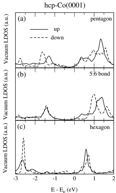
FIG. 5: Calculated spin-resolved vacuum LDOS at 5 Å above the  $C_{60}$  molecule deposited on hcp-Co(001) surface with various adsorption sites: (a) a pentagon ring, (b) a 5:6 bond, (c) a hexagon ring. Spin up/down curves are shown by solid/dashed lines.
