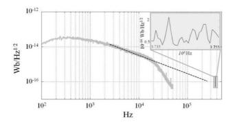
**Figure 4.** Flux sensitivity of the double-D channel. PSD of the noise measured with PowerLab 16/30 for the double-D coupled to the MS is reported from  $100\,\mathrm{Hz}$  to  $50\,\mathrm{kHz}$ . The 1/f trend of the sensor noise is extrapolated to frequencies larger than the A/D low pass filter at  $20\,\mathrm{kHz}$ . The inset shows the noise level measured by the NMR console in a narrow band across the NMR working frequency, which is above the 1/f corner.
