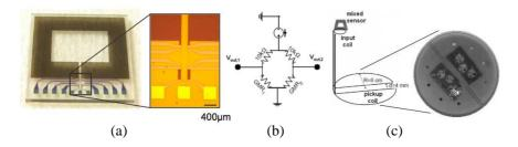
Figure 2. The superconducting NMR detector. (a) A photograph of the MS chip including the YBCO loop with the constriction above which the GMR yokes are placed (inset). (b) A schematic drawing of the read-out bridge, including two GMR yokes and two resistors. (c) The wire-wound double-D coil placed on a spherical fiberglass support, connected to an input coil tightly wound on the top of the YBCO loop.
