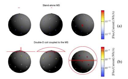
**Figure 5.** Spatial sensitivity of (a) the stand-alone MS and (b) the double-D set-up. The normalized flux generated by each coil through the sensor is coded in colour. Three projections of the calibrator sphere are shown together with the geometry of the stand-alone MS and the double-D coil.
