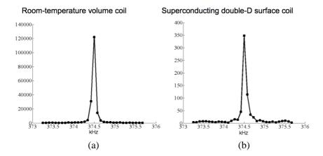
Figure 7. NMR spectra. NMR signal of the doped water phantom measured using (a) the volume room-temperature coil and (b) the double-D coil. The SNR with the double-D surface coil is  $\approx 182$ , with the volume resonant coil SNR  $\approx 776$ .
