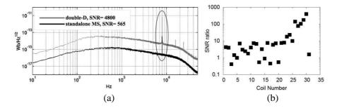
**Figure 6.** Comparison between the SNR of the stand-alone MS and the double-D set-up. (a) PSD of the magnetic flux through the stand-alone MS (black) and the double-D coil (grey) for equatorial coil number 25. (b) Ratio of the double-D and the stand-alone MS SNR as a function of the calibrator coil position.
