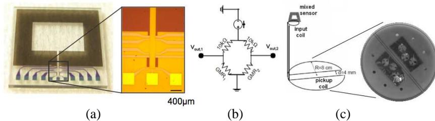
**Figure 2.** The superconducting NMR detector. (a) A photograph of the MS chip including the YBCO loop with the constriction above which the GMR yokes are placed (inset). (b) A schematic drawing of the read-out bridge, including two GMR yokes and two resistors. (c) The wire-wound double-D coil placed on a spherical fiberglass support, connected to an input coil tightly wound on the top of the YBCO loop.
