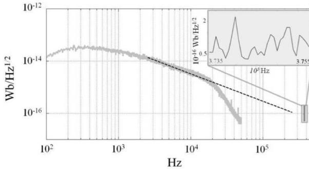
**Figure 4.** Flux sensitivity of the double-D channel. PSD of the noise measured with PowerLab 16/30 for the double-D coupled to the MS is reported from 100 Hz to 50 kHz. The  $1/f$  trend of the sensor noise is extrapolated to frequencies larger than the A/D low pass filter at 20 kHz. The inset shows the noise level measured by the NMR console in a narrow band across the NMR working frequency, which is above the  $1/f$  corner.
