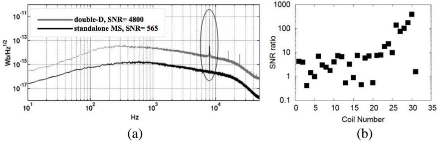
**Figure 6.** Comparison between the SNR of the stand-alone MS and the double-D set-up. (a) PSD of the magnetic flux through the stand-alone MS (black) and the double-D coil (grey) for equatorial coil number 25. (b) Ratio of the double-D and the stand-alone MS SNR as a function of the calibrator coil position.
