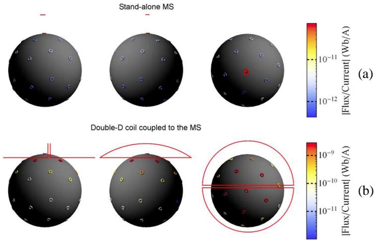
**Figure 5.** Spatial sensitivity of (a) the stand-alone MS and (b) the double-D set-up. The normalized flux generated by each coil through the sensor is coded in colour. Three projections of the calibrator sphere are shown together with the geometry of the stand-alone MS and the double-D coil.
