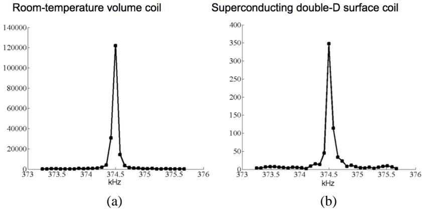
**Figure 7.** NMR spectra. NMR signal of the doped water phantom measured using (a) the volume room-temperature coil and (b) the double-D coil. The SNR with the double-D surface coil is  $\approx 182$ , with the volume resonant coil SNR  $\approx 776$ .
