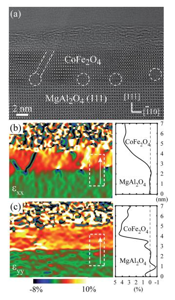
FIG. 2. HRTEM image of a CoFe<sub>2</sub>O<sub>4</sub>(111) film on MgAl<sub>2</sub>O<sub>4</sub>(111) (a). Dashed circles indicate dislocations, and the parallel dashed lines mark an antiphase boundary. The geometrical phase analysis is shown for the inplane deformation  $\varepsilon_{xx}$  (b) and the out-of-plane deformation  $\varepsilon_{yy}$  (c). Profile of the deformation in dashed rectangle is reported for each direction.
