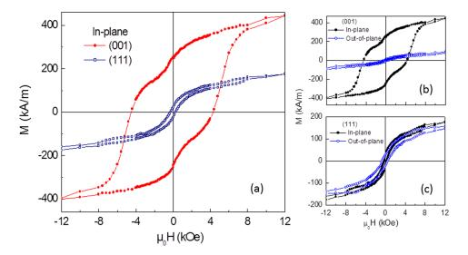
FIG. 3. (a) In-plane magnetic hysteresis loops at 300 K of a  $CoFe_2O_4$  (5 nm) film grown on MgAl<sub>2</sub>O<sub>4</sub>(100) and MgAl<sub>2</sub>O<sub>4</sub>(111). In-plane and out-ofplane hysteresis loops of the film on MgAl<sub>2</sub>O<sub>4</sub>(001) (b) and MgAl<sub>2</sub>O<sub>4</sub>(111) (c). In-plane hysteresis loops have been obtained along the [010] direction for CoFe<sub>2</sub>O<sub>4</sub>(001) and [-110] direction for CoFe<sub>2</sub>O<sub>4</sub>(111).
