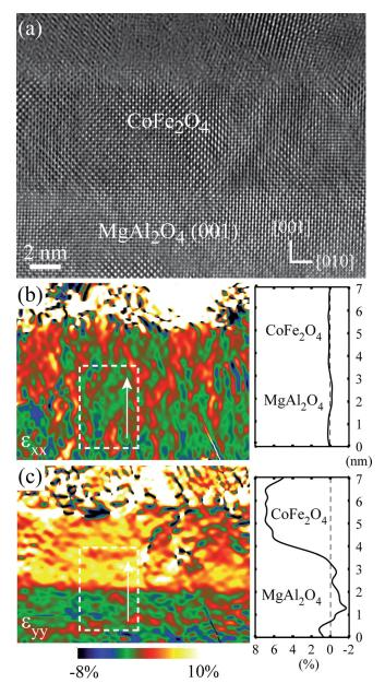
FIG. 1. HRTEM image of a CoFe<sub>2</sub>O<sub>4</sub>(001) film deposited on MgAl<sub>2</sub>O<sub>4</sub>(001) (a) with the corresponding geometrical phase analysis for the in-plane deformation  $\varepsilon_{xx}$  (b) and the out-of-plane deformation  $\varepsilon_{yy}$  (c). Profile of the deformation in dashed rectangle is reported for each direction.
