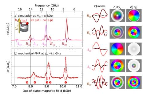
Fig. 1.5 Panel (a) is the simulated spectral response to an orthoradial excitation field  $h_1 \propto -\sin\phi \hat{x} + \cos\phi \hat{y}$ . Panel (b) is the experimental spectrum measured by mechanical-FMR for an RF current excitation. Panels (c)–(e) show the simulated precession patterns of the eigen-vectors
