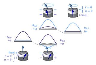
Fig. 1.3 Schematic representation of the coupled dynamics between two different magnetic disks. When the two disks are dynamically coupled through the dipolar interaction, the binding state *B* corresponds to the two layers oscillating in anti-phase at  $\omega_B$ , with the precession occurring mostly in the thick layer, whereas the anti-binding state *A* corresponds to the layers oscillating in phase at  $\omega_A$ , with the precession mostly in the thin layer
