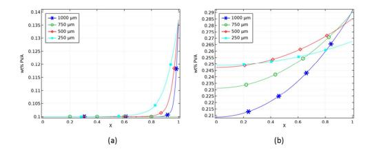
PVA concentration profiles for increasing initial solution thickness; (a) just before the composition path enters the diphasic region; (b) just before the composition path leaves the diphasic region - Ti = 25 °C, Tf = 80 °C, RH = 50, Temperature ramp = 35 °C/min Fig. 12 170x73mm (150 x 150 DPI)
