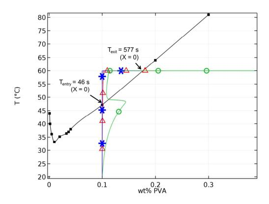
Composition path simulated by the model - Ti = 20 °C, Tf = 60 °C, RH = 50%, Tramp = 35 °C/min, Casting thickness = 1 mm Fig. 5 160x120mm (220 x 220 DPI)
