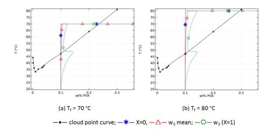
Composition path simulated by the model - Ti = 20 °C, Tf = 70 and 80 °C, RH = 50%, Tramp = 35 °C/min, Casting thickness = 1 mm Fig. 8 167x88mm (150 x 150 DPI)
