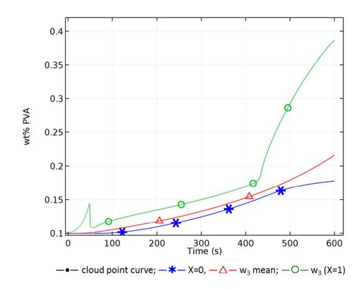
Weight fraction of PVA versus time - Ti = 20 °C, Tf = 60 °C, RH = 50%, Tramp = 35 °C/min, Casting thickness = 1 mm Fig. 7 143x119mm (150 x 150 DPI)
