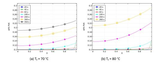
Simulated PVA concentration profiles prior to phase inversion (20 s, 45 s) and when the composition path is in the diphasic region (60 to final time step just before leaving the diphasic region) - Ti = 20 °C, Tf = 70 °C and 80 °C, RH = 50%, Tramp = 35 °C/min, casting thickness = 1 mm Fig. 9
