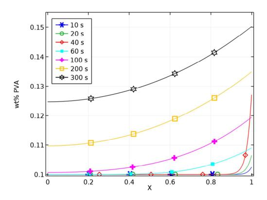
Concentration profiles simulated by the model - Ti = 20 °C, Tf = 60 °C, RH = 50%, Tramp = 35 °C/min, Casting thickness = 1 mm Fig. 6 135x101mm (150 x 150 DPI)
