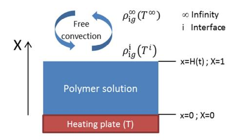
Schematic of LCST-TIPS process Fig. 2 95x70mm (150 x 150 DPI)
