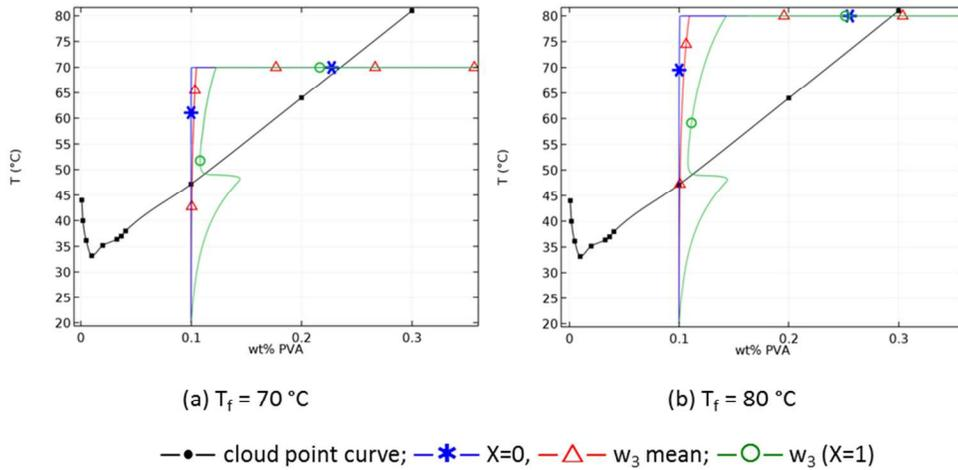
Composition path simulated by the model -  $T_i = 20\text{ }^\circ\text{C}$ ,  $T_f = 70$  and  $80\text{ }^\circ\text{C}$ ,  $RH = 50\%$ ,  $Tramp = 35\text{ }^\circ\text{C}/\text{min}$ ,
