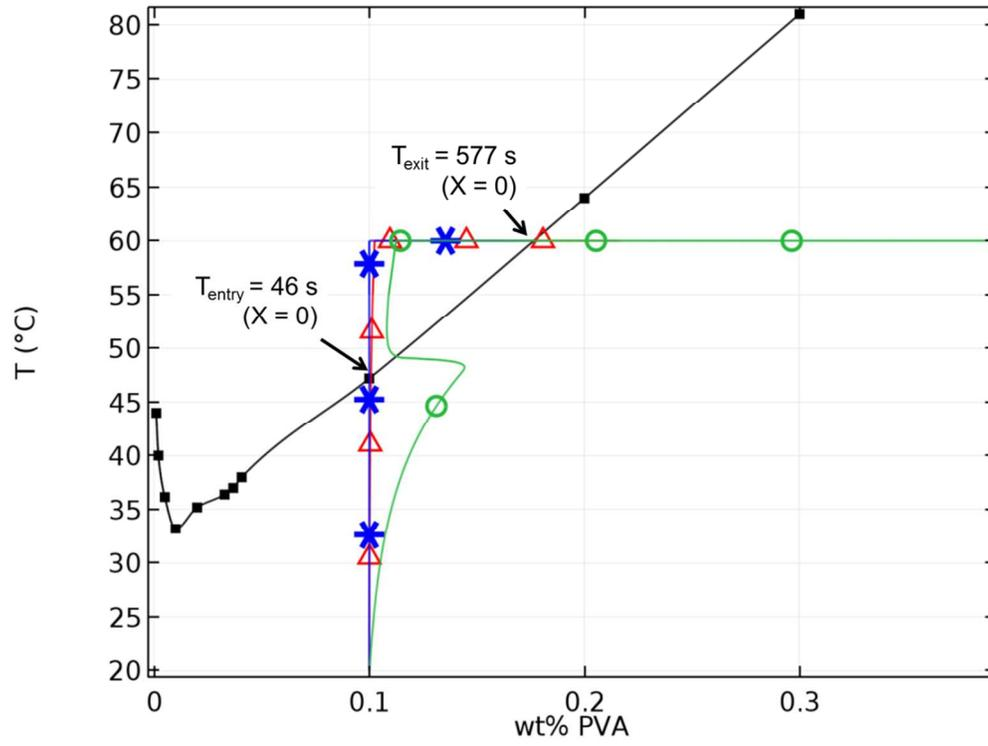
Composition path simulated by the model -  $T_i = 20\text{ }^\circ\text{C}$ ,  $T_f = 60\text{ }^\circ\text{C}$ ,  $RH = 50\%$ ,  $Tramp = 35\text{ }^\circ\text{C}/\text{min}$ , Casting thickness = 1 mm
