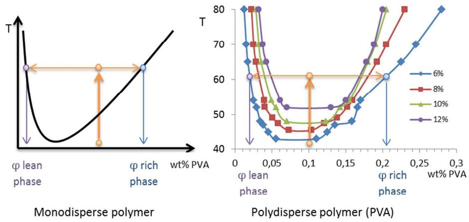
Phase diagram and coexistence curves pour PVA versus monodisperse polymer
