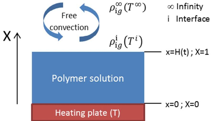
Schematic of LCST-TIPS process
