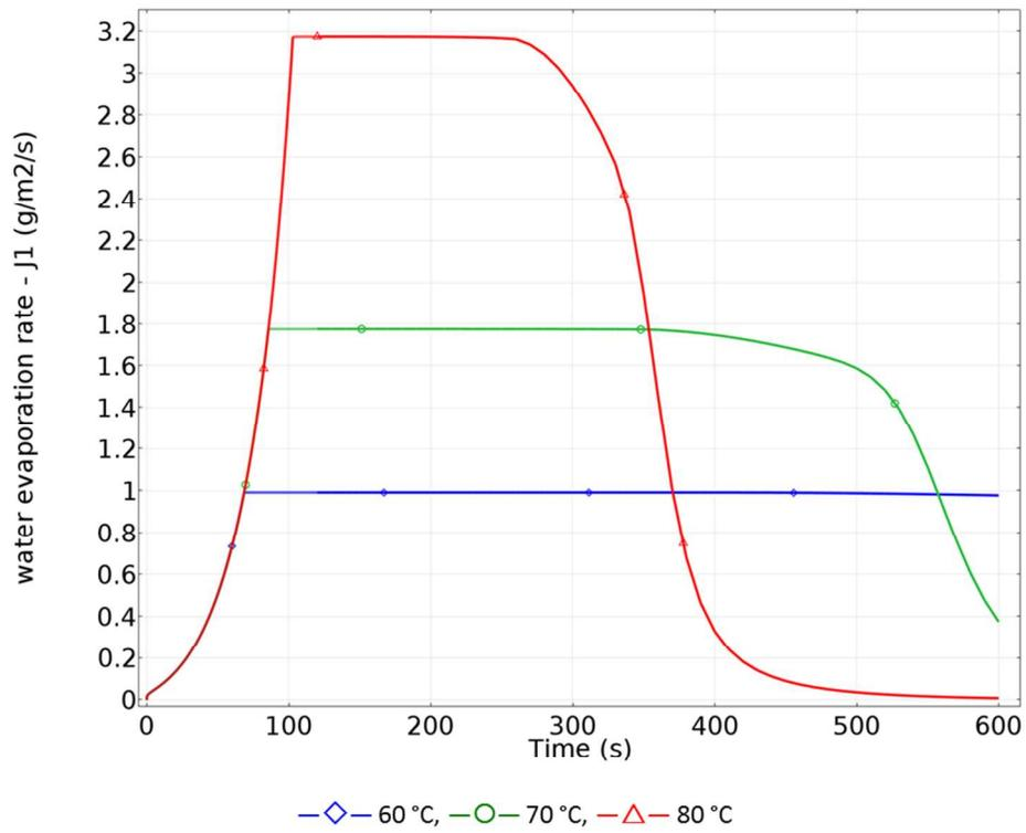
Water evaporation flux -  $T_i = 20\text{ }^\circ\text{C}$ ,  $T_f = 60\text{ }^\circ\text{C}$ ,  $70\text{ }^\circ\text{C}$  and  $80\text{ }^\circ\text{C}$ ,  $RH = 50\%$ ,  $Tramp = 35\text{ }^\circ\text{C}/\text{min}$ , casting thickness = 1 mm
