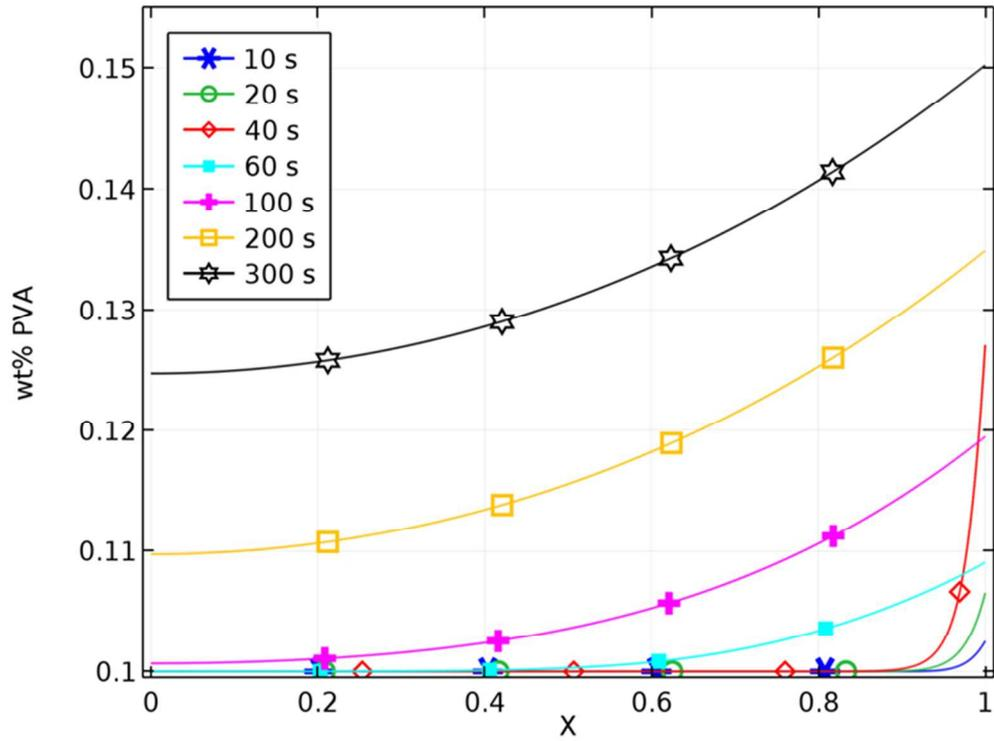
Concentration profiles simulated by the model -  $T_i = 20\text{ }^\circ\text{C}$ ,  $T_f = 60\text{ }^\circ\text{C}$ ,  $RH = 50\%$ ,  $Tramp = 35\text{ }^\circ\text{C}/\text{min}$ ,
