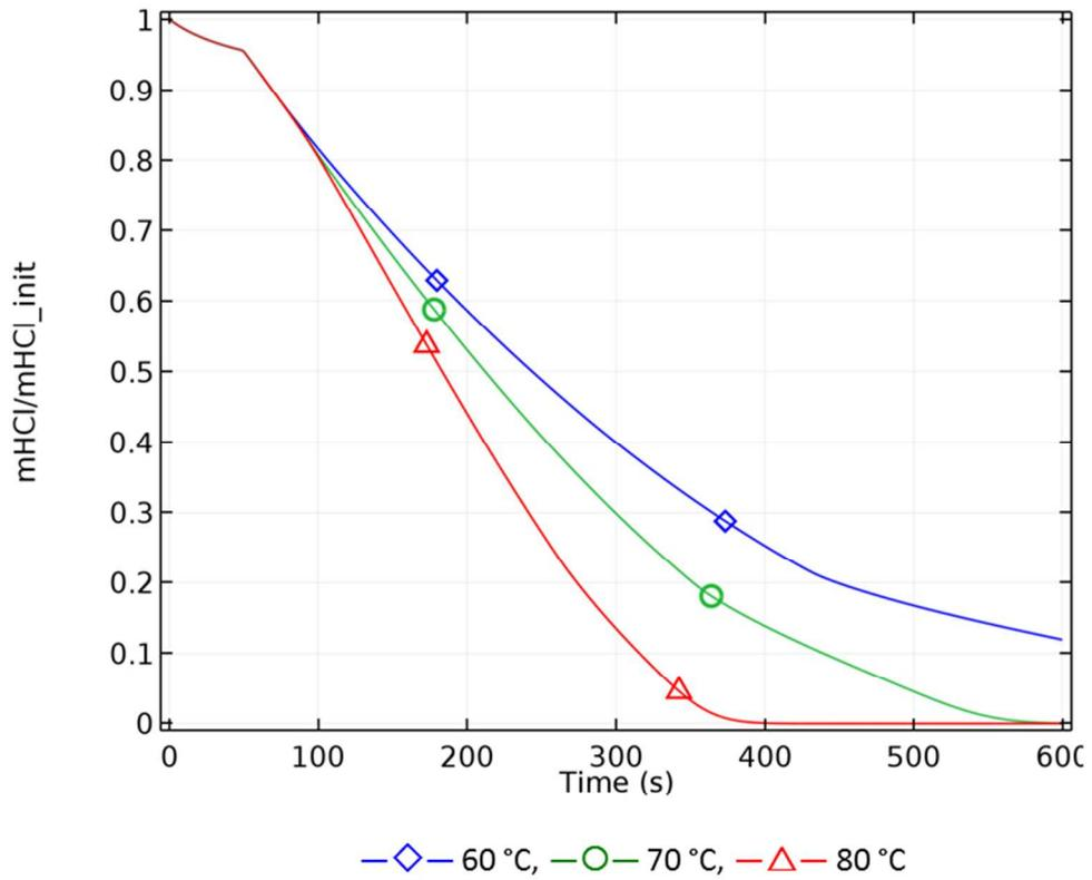
Loss of HCl during membrane formation – ratio between HCl mass at time t to initial HCl mass -  $T_i = 20\text{ }^\circ\text{C}$ ,
