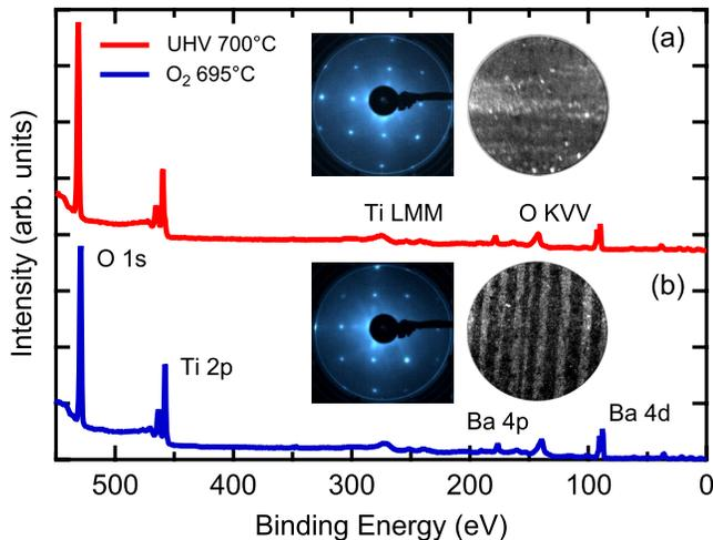
FIG. 1 (color online). XPS survey spectra of BTO(001) after (a) annealing in UHV at 700 °C and (b) annealing in  $6 \times 10^{-6}$  mbar of oxygen at 700 °C. The insets show the corresponding LEED (left) and PEEM (right) images. The PEEM field of view is  $65 \mu\text{m}$ .
