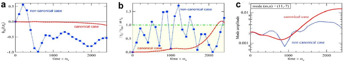
Fig. 1. In both canonical and non-canonical cases ( $\rho^{\star} = 10^{-2}$ ): (a) time evolution of the  $(m, n) = (0, 0)$  mode of the electric potential (b) ratio of the  $\mathbf{E} \times \mathbf{B}$  shearing rate over a rough estimate of the linear growth rate (c) time evolution of the most unstable mode.
