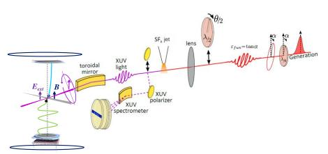
Fig. 3 Schematic of the experimental set-up combining the HHG PLFA beamline and the electron-ion 3D-momentum spectrometer.
