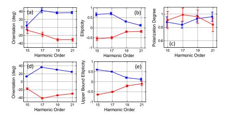
Fig. 8 First row: MP (a) Orientation of the polarization ellipse ( $\psi$ ) relative to the reference direction of the driving IR laser (b) measured ellipticity ( $\varepsilon$ ) (c) polarization degree, for  $\varepsilon_{fun} \approx 0.23$  (blue dots) and  $\varepsilon_{fun} \approx -0.17$  (red dots).
