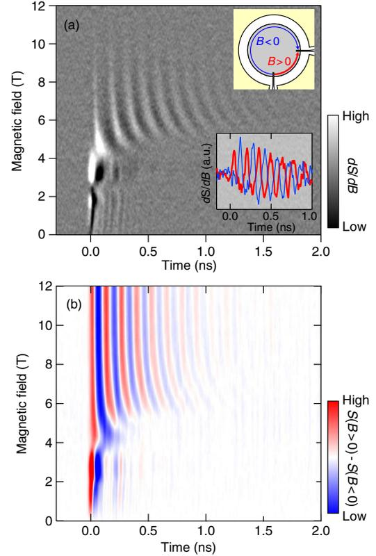
FIG. 3 (color online). Results of time domain measurement. (a) Differential signal ( $dS/dB$ ) of the 200- $\mu\text{m}$  sample a function of time and  $B$ . Inset shows  $dS/dB$  at  $B = 6.5$  T (red thick trace) and  $B = -6.5$  T (blue trace). The chirality of the EMP orbital motion is counterclockwise (clockwise) for positive (negative)  $B$ . (b)  $S(B > 0) - S(B < 0)$  for the 200- $\mu\text{m}$  sample.
