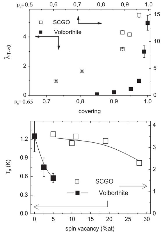
Fig. 4. Top panel: dependence on dilution of the relaxation rate on the dynamical plateau for a kagomé bilayer (SCGO) [7,6] and volborthite (this study). The  $x$  axes have been normalized by the percolation threshold for each lattice. Bottom panel: dependence on dilution of the transition temperature obtained by SQUID measurements [11,13] in the same compounds.
