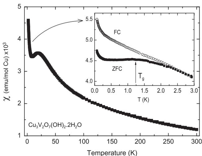
Fig. 1. Macroscopic susceptibility versus temperature in pure volborthite in 100 Oe. Inset: zoom on the very low temperature data. The upturn below  $T \simeq 200$  mK is an artifact due to few ppm magnetic impurities in the grease used to ensure thermalization of the powder sample.
