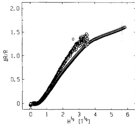
Fig. 3.  $\Delta R/R = [R(H) - R(0)]/R(0)$  versus  $H^{1/2}$  at  $T = 60 \text{ mK}$  in constant field of  $7 \text{ T}$  ( $\diamond$ ), and for 2 pulsed field experiments.
