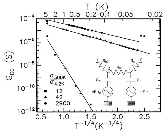
FIG. 1. Mott's law for samples with resistivity ratios  $R(4.2 \text{ K})/R(300 \text{ K})$  of 3000, 40, and 12. The corresponding values of  $T_0$  are 2940, 2.6, and 1.2 K. Inset: equivalent impedance network at finite temperature.
