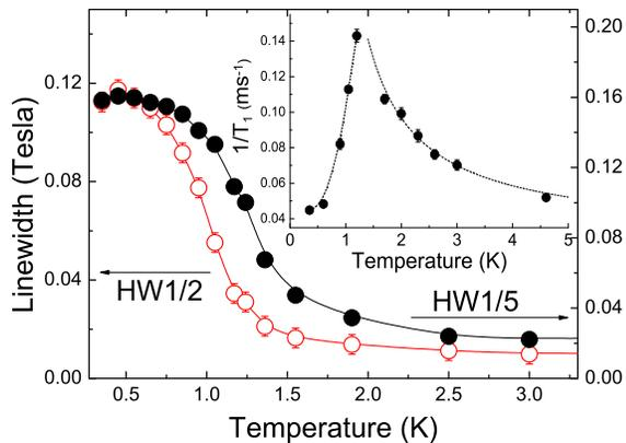
FIG. 3: Half widths of the NMR spectra measured at 1/2 (HW1/2, open symbols) and 1/5 (HW1/5, full symbols) of the maximum height. Inset :  $T$ -dependence of the  $^{51}\text{V}$  spin-lattice relaxation rate ( $1/T_1$ ) measured at the maximum intensity of the spectra ( $H=1.85$  T). Lines are guides for the eye.
