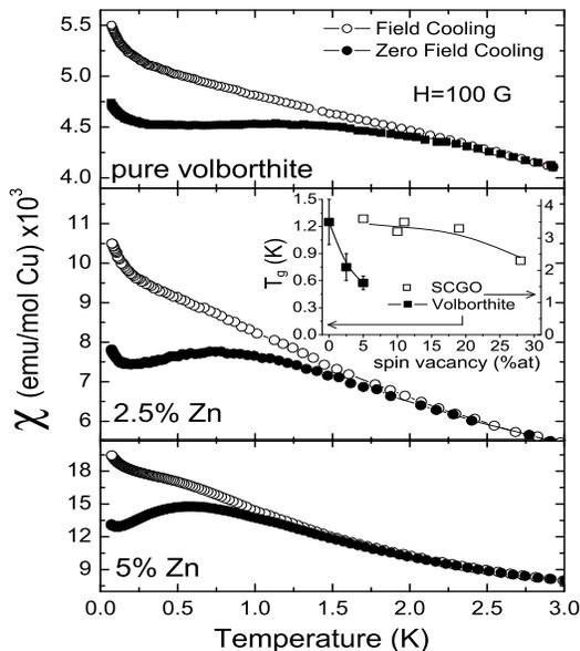
FIG. 1: SQUID dc susceptibility in  $\text{Cu}_{3(1-x)}\text{Zn}_{3x}\text{V}_2\text{O}_7(\text{OH})_2 \cdot 2\text{H}_2\text{O}$  measured after two cooling protocols, with (open symbols) and without (full symbols) a 100 Oe applied field. Inset: comparison of  $T_g$  versus  $S=0$  impurity dilution rate in volborthite and SCGO bilayer compounds.
