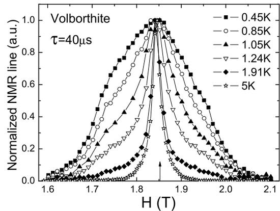
FIG. 2:  $^{51}\text{V}$  NMR spectra measured at 20.733 MHz as a function of the applied field. For clarity, the spectra have been normalized to their maximum value. The vertical arrow shows the position  $H_0$  of the unshifted reference line.
