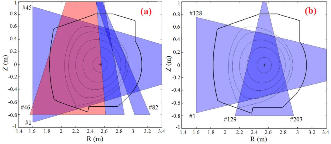
Figure 1. WEST plasma coverage of the (a) former Tore Supra diodes (b) new GEM based SXR cameras. The red part of the former viewing angle is lost due to the WEST upper divertor.
