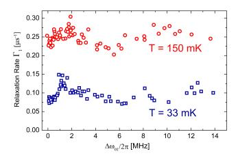
Figure 4: Frequency dependence of the relaxation rate  $\Gamma_1$  of Q4 in the vicinity of its optimal point at T=33mK (blue squares) and T=150mK (red circles), showing an increased relaxation rate caused by quasi-particles.
