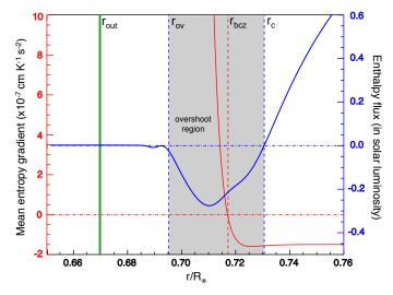
**Fig. 6.** Representation of the overshoot region defined between  $r_{\rm c}$ , the first zero of the enthalpy flux, and the point  $r_{\rm ov}$  below which the amplitude of the flux drops to 10% of its most negative value. The radius  $r_{\rm bcz}$  corresponds to the point where the mean entropy gradient changes sign. The green vertical line represents the positions of  $r_{\rm out}$  for  $\omega = 0.2$  mHz.
