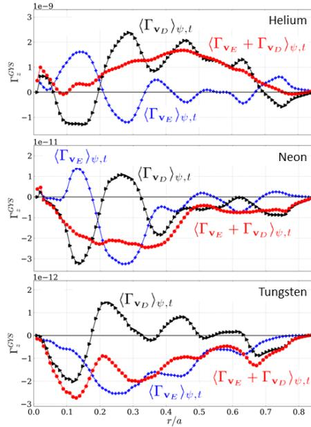
**Figure 8.** Time and flux-surface average of the radial impurity flux in D-Helium, D-Neon and D-Tungsten simulations. The total flux (red) is decomposed into its electric (blue) and magnetic (black) drift components.
