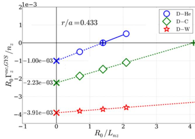
**Figure 4.** Detail of the method used to retrieve the pinch velocity of 3 impurities (He, C and W) in a deuterium plasma (no temperature gradient). The slope provides the diffusion coefficient, the intersection with the  $y$ -axis gives the pinch velocity. Intersection points with the  $x$ -axis correspond to the expected equilibrium gradient of the impurity density profiles as a result of the sole main ion density gradient (density peaking).
