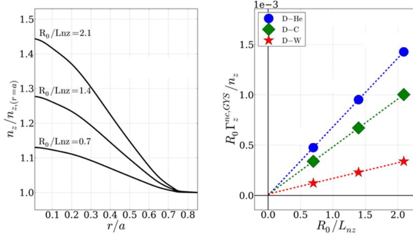
**Figure 2.** Left: the 3 impurity density profiles considered for GYSELA simulations. Right: the time averaged neoclassical flux computed for each of these profiles is plotted versus the normalized density gradient in the case of 3 impurities (He, C and W) in a deuterium plasma. The slope gives the neoclassical diffusion coefficient.
