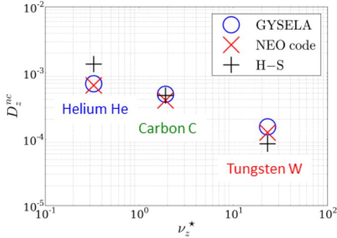
**Figure 3.** Diffusion coefficient of 3 impurities (He, C and W) in a deuterium plasma versus the impurity collisionality  $\nu_z^*$ . The GYSELA results (o) are compared with the values predicted by Hirshman-Sigmar [45] (+) and the ones obtained with the NEO code (x).
