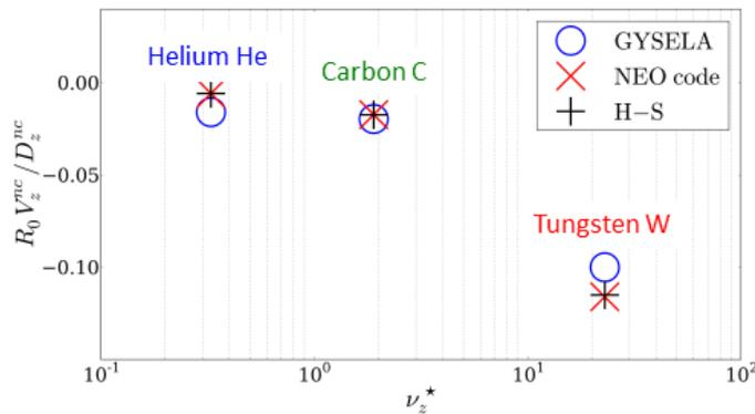
**Figure 5.** Normalized pinch velocity of 3 impurities (He, C and W) in a deuterium plasma versus the impurity collisionality  $\nu_z^*$ . The GYSELA results (o) are compared with the values predicted by Hirshman-Sigmar (+) and the ones obtained with the NEO code (x).
