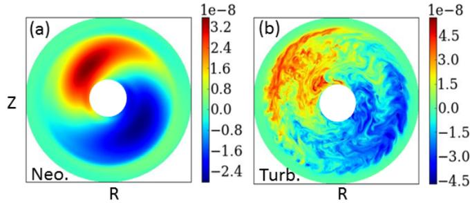
**Figure 12.** Instantaneous poloidal cross-sections of tungsten density fluctuations  $\delta N_W = N_W - \langle N_W \rangle_{FS}$  (with  $\langle \dots \rangle_{FS}$  the flux-surface average) for the 2 reduced simulations in the case of a deuterium-tungsten plasma.
