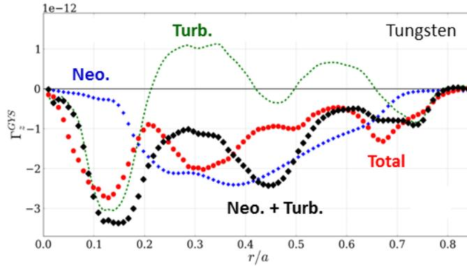
**Figure 10.** Time-averaged radial tungsten flux in neoclassical (blue), turbulent (green) and full (red) simulations. The sum of the fluxes of the neoclassical and turbulent simulations is shown in black.
