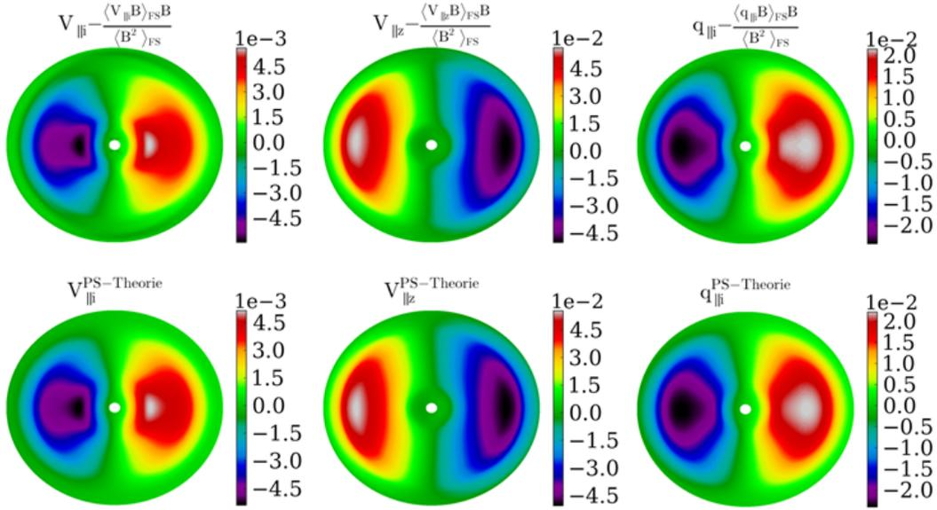
**Figure 7.** Top row: poloidal fluctuations of the actual parallel velocities and flux obtained with GYSELA. Bottom row: same quantity computed from the radial gradients (cf. eqs.(36-38)). The agreement between theory and modeling looks satisfactory.
