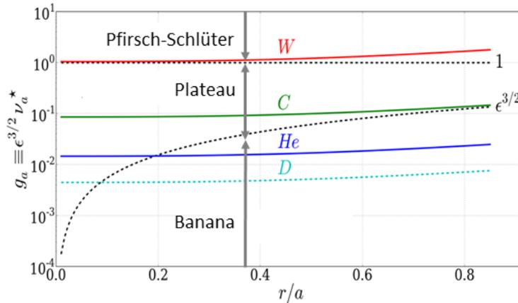
**Figure 1.** For a given radial profile of deuterium collisionality (blue dashed line), corresponding profiles of the collisionality of 3 trace impurities: helium (He), carbon (C) and tungsten (W,  $Z_W = 40$  here). The limits of the three collisionality regimes (banana, plateau, Pfirsch-Schlüter) are also displayed.
