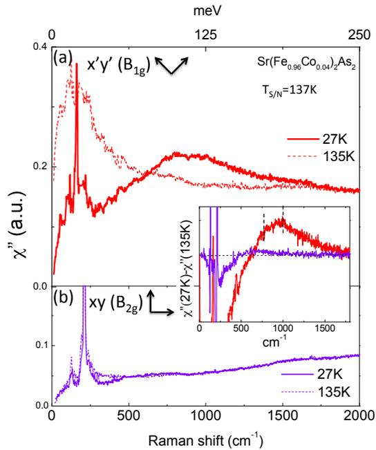
FIG. 2: Raman spectra in  $x'y'$  ( $B_{1g}$ ) and  $xy$  ( $B_{2g}$ ) symmetries for  $\text{Sr}(\text{Fe}_{1-x}\text{Co}_x)_2\text{As}_2$  ( $T_N=137$  K) using 2.33 eV excitation energy. The inset shows the subtraction between the response at low temperature (27 K) and the response at  $\sim T_N$  for both symmetries. The dotted lines highlight the positions of the two kinks observed at  $\sim 750$  and  $1000$   $\text{cm}^{-1}$  in the  $x'y'$  spectrum.
