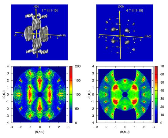
FIG. 2. (Color online) Neutron diffuse scattering maps in reciprocal space at 0.16 K in  $\text{Tb}_2\text{Ti}_2\text{O}_7$  with a field applied along [1 $\bar{1}$ 0]. (Top) 3D equal intensity surfaces for a magnetic field of 1 (left) and 4 T (right). (Bottom) Cuts in the (hhl) plane of the maps at 1 (left) and 4 T (right).
