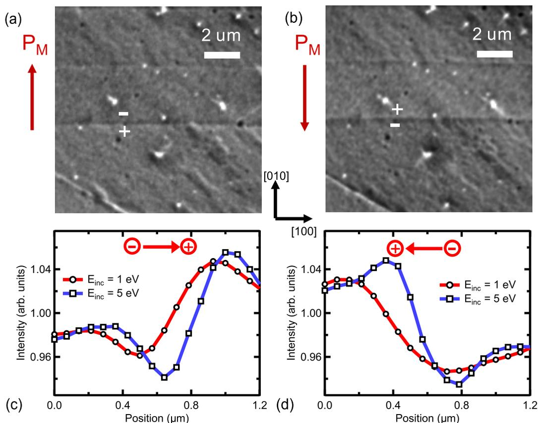
**Figure 4** | LEEM images of sample surface before (a) and after (b) switching, the field of view is  $30 \mu\text{m}$ . Intensity profiles extracted from LEEM images acquired using 1 eV (round, red symbols) and 5 eV (square, black symbols) along  $[010]$  across a domain wall before (c) and after (d) switching. The deduced electric dipole across the wall is shown by the plus and minus signs.
