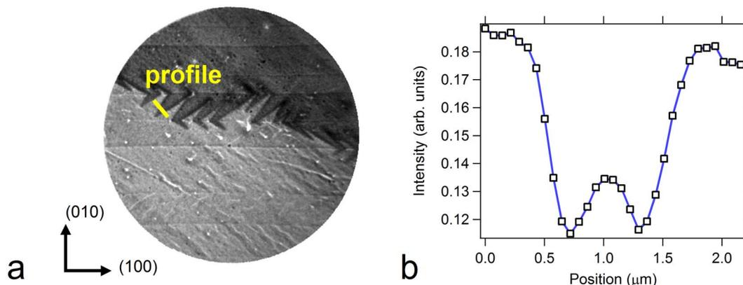
**Figure 7** | (a) Electron image of  $\text{BaTiO}_3$  surface during switching, the thick yellow line shows where the intensity profile was taken (b) Intensity profile across needle domain perpendicular to the polar direction.
