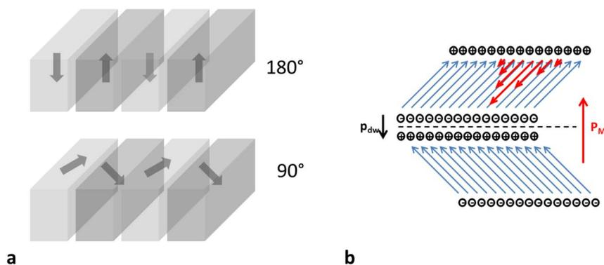
**Figure 1** | (a) Schematic of  $180^\circ$  (top) and  $90^\circ$  (bottom) domain walls in  $\text{BaTiO}_3(001)$ . In the latter the polarization directions are in-plane (b)  $90^\circ$  domain walls between in-plane polarized domains showing net macroscopic polarization and domain wall dipoles. The thicker (red online) arrows represent the switched polarization in the form of a needle, described below.
