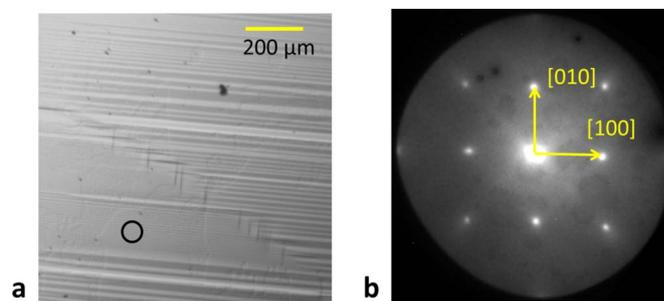
**Figure 2** | (a) Optical micrograph of the  $\text{BaTiO}_3$  surface showing domain ordering on a macroscopic scale. For comparison, the size of the electron beam is indicated by the black circle. (b)  $(1 \times 1)$  LEED pattern using a primary electron energy of 35 eV.
