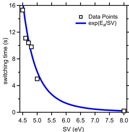
**Figure 5** | Switching time (squares) as a function of sample bias. Below 4.3 eV the polarization does not switch, at 8 eV the switching is below 0.1 seconds. The blue line is an exponential fit to the data.
