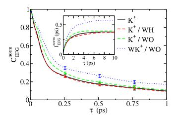
FIG. 2. Normalized correlation function  $C_{EFG}^{norm}$  and their integrals (inset) of the EFG at the nucleus site of an aqueous potassium ion. In addition to the real system, we consider the effect of isotopic substitutions by doubling the mass of the oxygen (WO) or hydrogen (WH) of water molecules. In the last model (WK<sup>+</sup>), the mass of the ion is infinite. Error bars indicate standard deviations over five independent trajectories.
