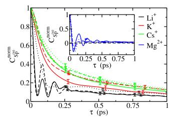
FIG. 5. Normalized correlation functions of different functions of the family defined by Eqs. (9) and (10):  $\mathbf{S}_{-1}^{(1)}$  (continuous line),  $\mathbf{S}_{0}^{(2)}$  (dotted line), and  $\mathbf{S}_{4}^{(2)}$  (dashed line) around different alkali (main figure) and magnesium (inset) cations in water at infinite dilution. Error bars indicate standard deviations over five independent trajectories.
