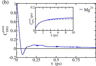
FIG. 1. Normalized electric field gradient autocorrelation functions,  $C_{EFG}^{norm}$ , and their integrals (inset) for aqueous ions with normal (full lines) and infinite (dashed lines) mass at infinite dilution: (a) Li<sup>+</sup>, K<sup>+</sup>, and Cs<sup>+</sup> and (b) Mg<sup>2+</sup>. Error bars indicate standard deviations over five independent trajectories.
